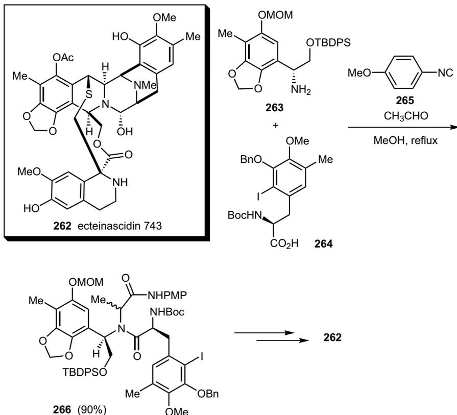
**Scheme 12.37.** Synthesis of ecteinascidin 743 using a Ugi 4CR, by Fukuyama and co-workers [132] MOM = methoxymethyl, TBDPS = *t*-butyldiphenylsilyl, Boc = *t*-butoxycarbonyl, Bn = benzyl, PMP = *p*-methoxyphenyl.
