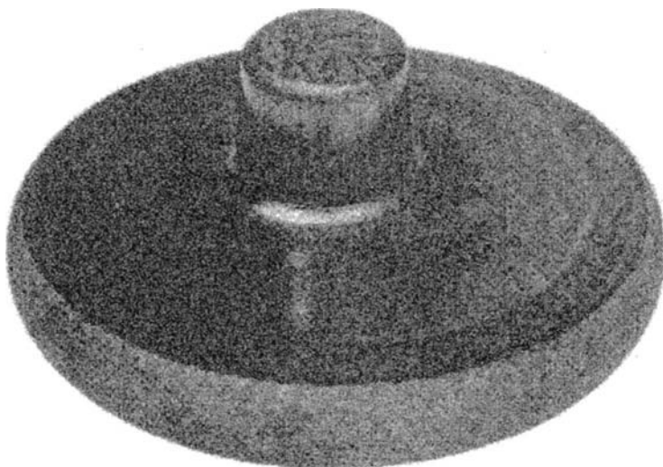
FIGURE 6.12 Deformed billet and spike.
