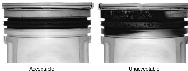
FIGURE 19.6 Detergents keep upper pistons clean.
