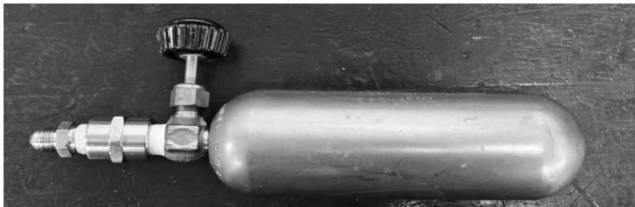
FIGURE 18.4 Monel cylinder ( V = 100 mL) with Monel valve. (For a color version of the figure, please see color plates.)
