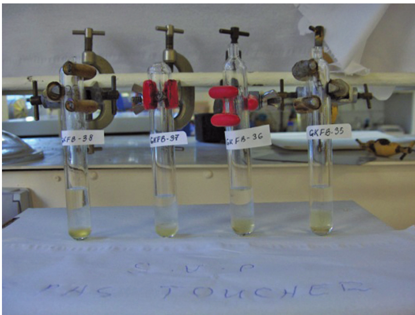
FIGURE 59.4 Picture of Carius tubes after the radical copolymerization of VDF with \alpha,\beta -difluoroacrylic acid.
