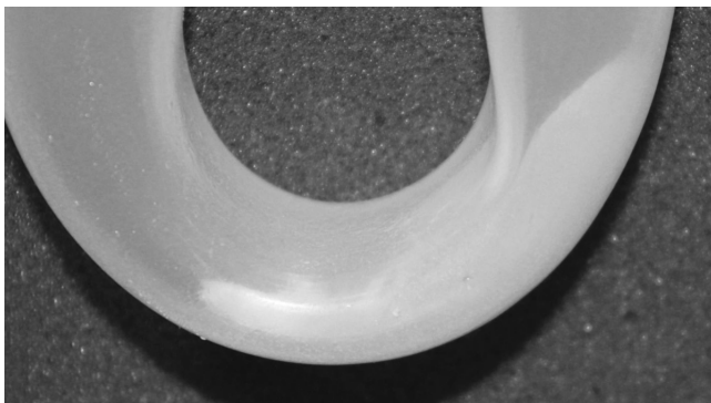
FIGURE 18.5 Teflon/FEP U-trap with solid \text{ReF}_6 . (For a color version of the figure, please see color plates.)
