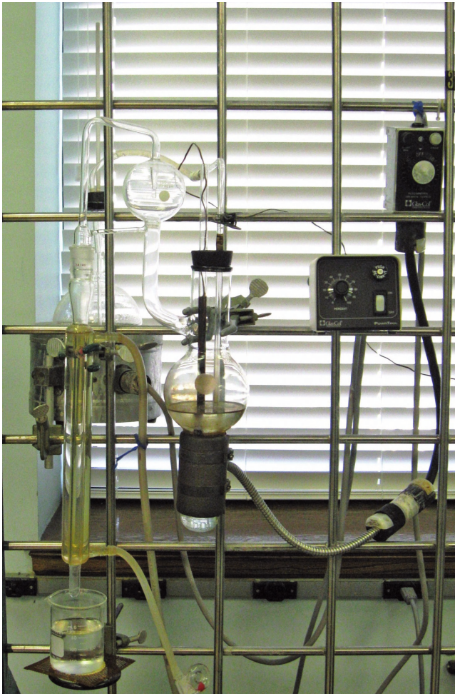
FIGURE 9.1 Setup for Willard-Winter Distillation Method.
