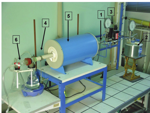
FIGURE 64.2 Sulfurization apparatus for preparing lanthanum sulfofluoride LaSF.
