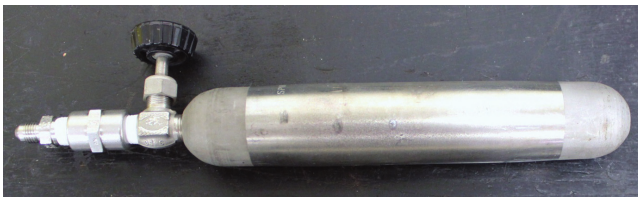
FIGURE 18.1 Stainless steel cylinder ( V = 175 \text{ mL} ) with stainless steel valve.
