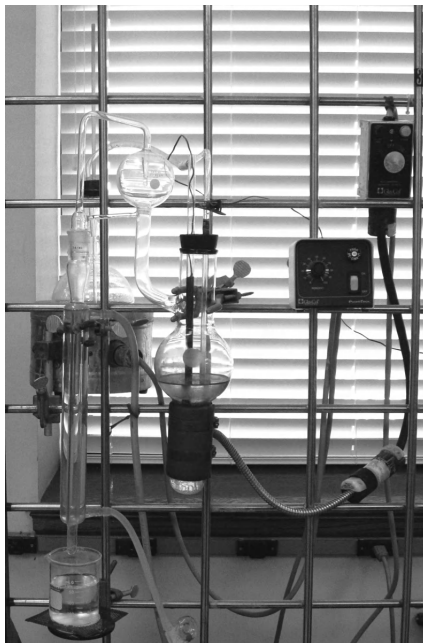
FIGURE 9.1 Setup for Willard–Winter distillation method. (For a color version of the figure, please see color plates.)
