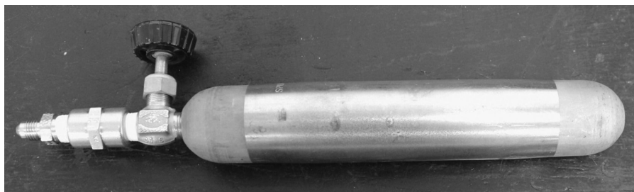
FIGURE 18.1 Stainless steel cylinder ( V = 175 \text{ mL} ) with stainless steel valve. (For a color version of the figure, please see color plates.)
