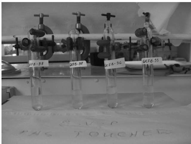
FIGURE 59.4 Picture of CTs after the radical copolymerization of VDF with \alpha,\beta -difluoroacrylic acid. (For a color version of the figure, please see color plates.)
