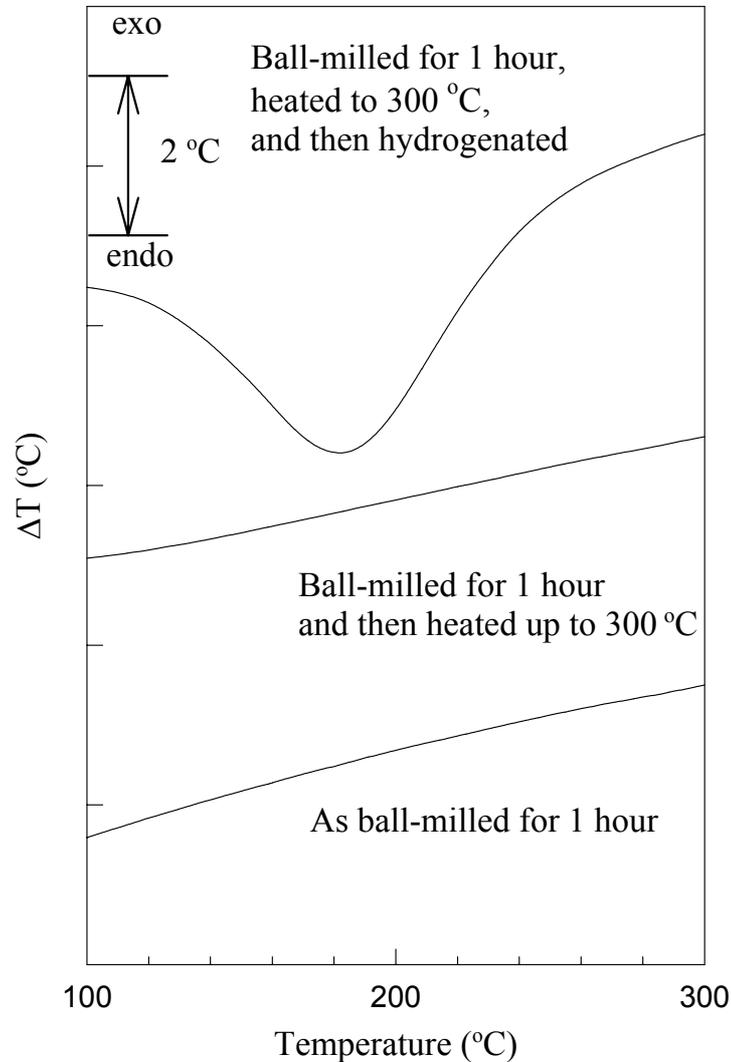
Figure 10. The DTA traces of pure  $\text{Zr}_{27}\text{Ti}_9\text{Ni}_{38}\text{V}_5\text{Mn}_{16}\text{Cr}_5$  ball-milled for 1 hour, ball-milled for 1 hour and then heated to 300 °C for 15 min, and ball-milled for 1 hour, heated to 300 °C, and then hydrogenated.
