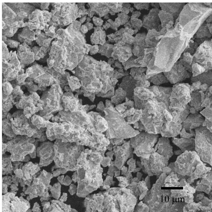
Figure 41. Morphology of pure  $\text{LaNi}_{4.85}\text{Sn}_{0.15}$  ball-milled for 6 hours.
