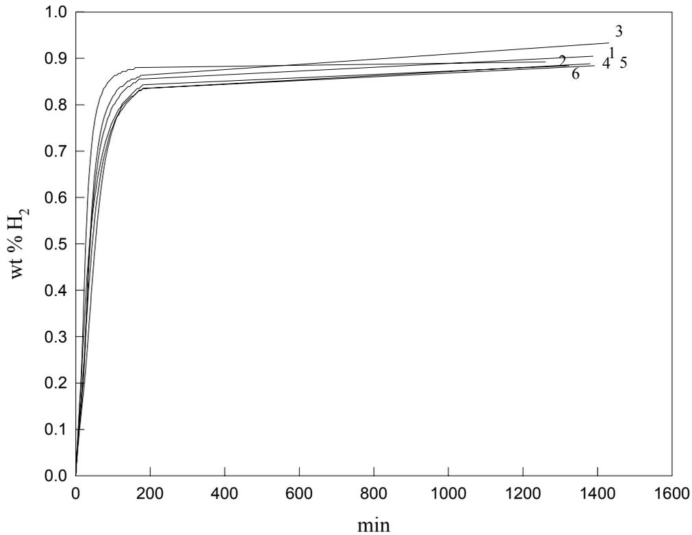
Figure 23. Hydrogenation behavior of  $\text{LiAlH}_4 + \text{Zr}_{27}\text{Ti}_9\text{Ni}_{38}\text{V}_5\text{Mn}_{16}\text{Cr}_5$  at 3.3-1.8 atm pressure at room temperature taken in 1:1 volume ratio and ball-milled for 6 hours. The numeral next to the curve indicates hydrogenation cycle number.
