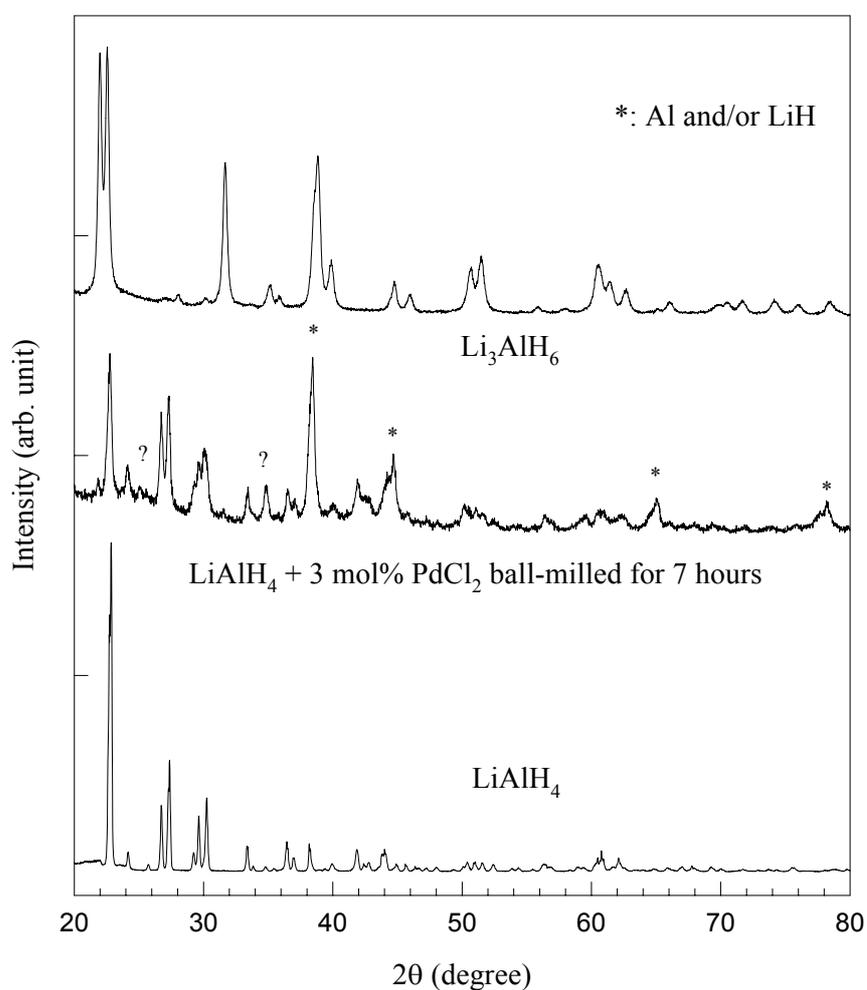
Figure 47. The XRD patterns of pure LiAlH<sub>4</sub> [21], LiAlH<sub>4</sub> + 3 mol% PdCl<sub>2</sub> ball-milled for 7 hours, and pure Li<sub>3</sub>AlH<sub>6</sub> [21].
