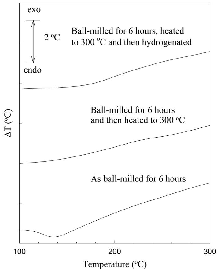
Figure 38. The DTA traces of LiAlH<sub>4</sub> + LaNi<sub>4.85</sub>Sn<sub>0.15</sub> taken in 1:1 volume ratio and ball-milled for 6 hours, ball-milled for 6 hours and then heated to 300 °C for 15 min, and ball-milled for 6 hours, heated to 300 °C, and then hydrogenated.
