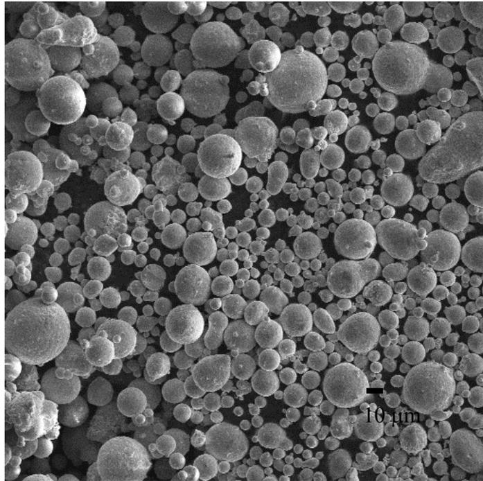
Figure 33. Morphology of annealed  $\text{LaNi}_{4.85}\text{Sn}_{0.15}$  (x 300).
