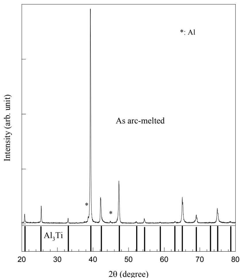
Figure 43. The XRD pattern of arc-melted Al<sub>3</sub>Ti.
