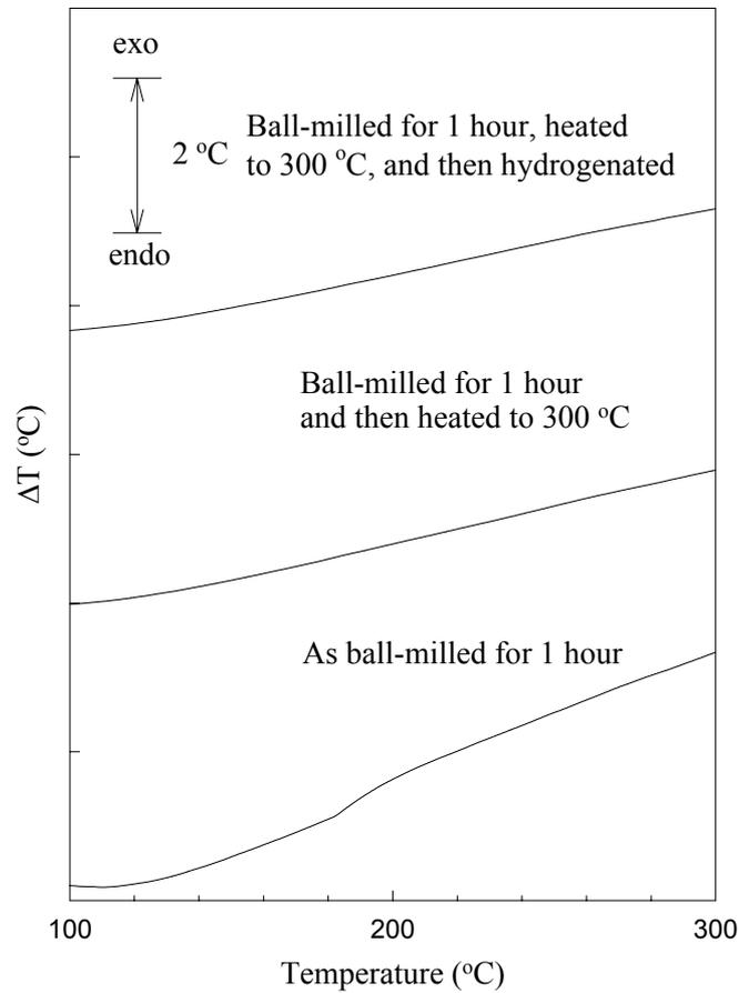
Figure 29. The DTA traces of pure  $\text{LaNi}_{4.85}\text{Sn}_{0.15}$  ball-milled for 1 hour, ball-milled for 1 hour and then heated to  $300\text{ }^{\circ}\text{C}$  for 15 min, and ball-milled for 1 hour, heated to  $300\text{ }^{\circ}\text{C}$ , and then hydrogenated.
