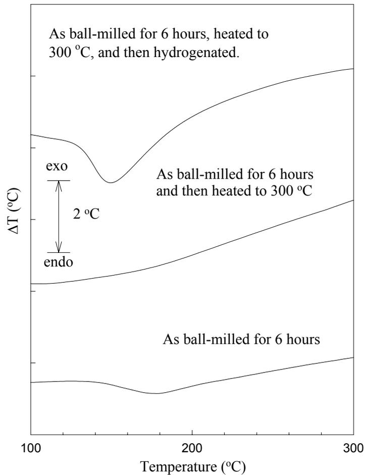
Figure 21. The DTA traces of  $\text{LiAlH}_4 + \text{Zr}_{27}\text{Ti}_9\text{Ni}_{38}\text{V}_5\text{Mn}_{16}\text{Cr}_5$  taken in 1:1 volume ratio and ball-milled for 6 hours, ball-milled for 6 hours and then heated to 300 °C for 15 min, and ball-milled for 6 hours, heated to 300 °C, and then hydrogenated.
