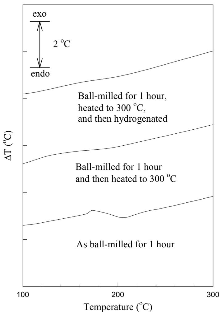
Figure 11. The DTA traces of  $\text{LiAlH}_4 + \text{Zr}_{27}\text{Ti}_9\text{Ni}_{38}\text{V}_5\text{Mn}_{16}\text{Cr}_5$  taken in 1:1 volume ratio and ball-milled for 1 hour, ball-milled for 1 hour and then heated to 300 °C for 15 min, and ball-milled for 1 hour, heated to 300 °C, and then hydrogenated.
