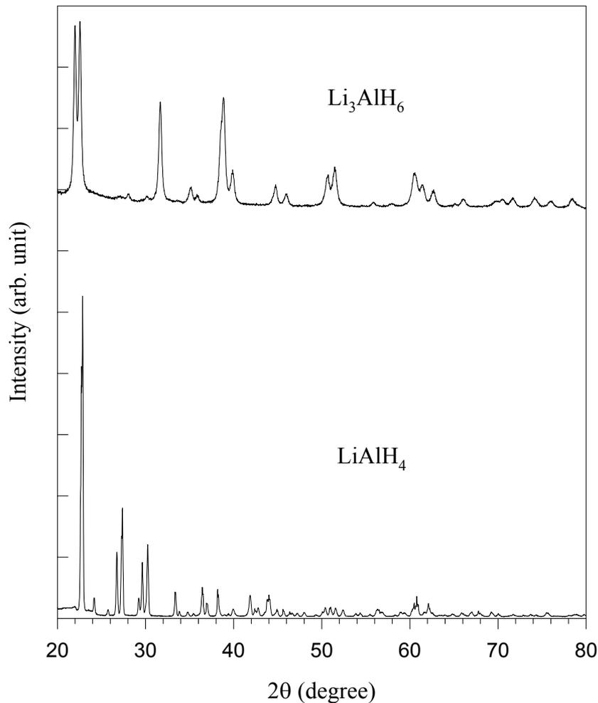
Figure 9. XRD patterns of  $\text{LiAlH}_4$  and  $\text{Li}_3\text{AlH}_6$  [21].
