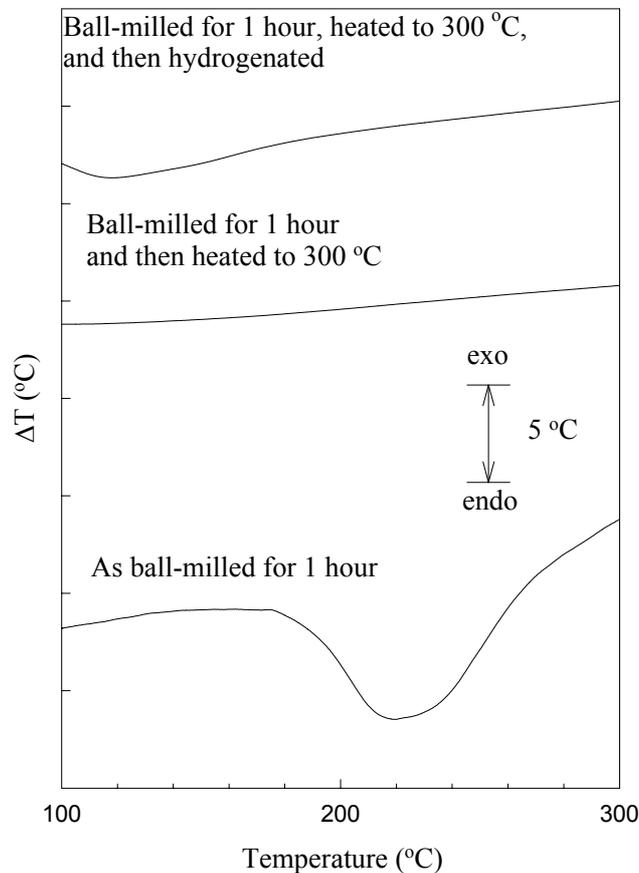
Figure 30. The DTA traces of  $\text{LiAlH}_4 + \text{LaNi}_{4.85}\text{Sn}_{0.15}$  taken in 1:1 volume ratio and ball-milled for 1 hour, ball-milled for 1 hour and then heated to 300 °C for 15 min, and ball-milled for 1 hour, heated to 300 °C, and then hydrogenated.
