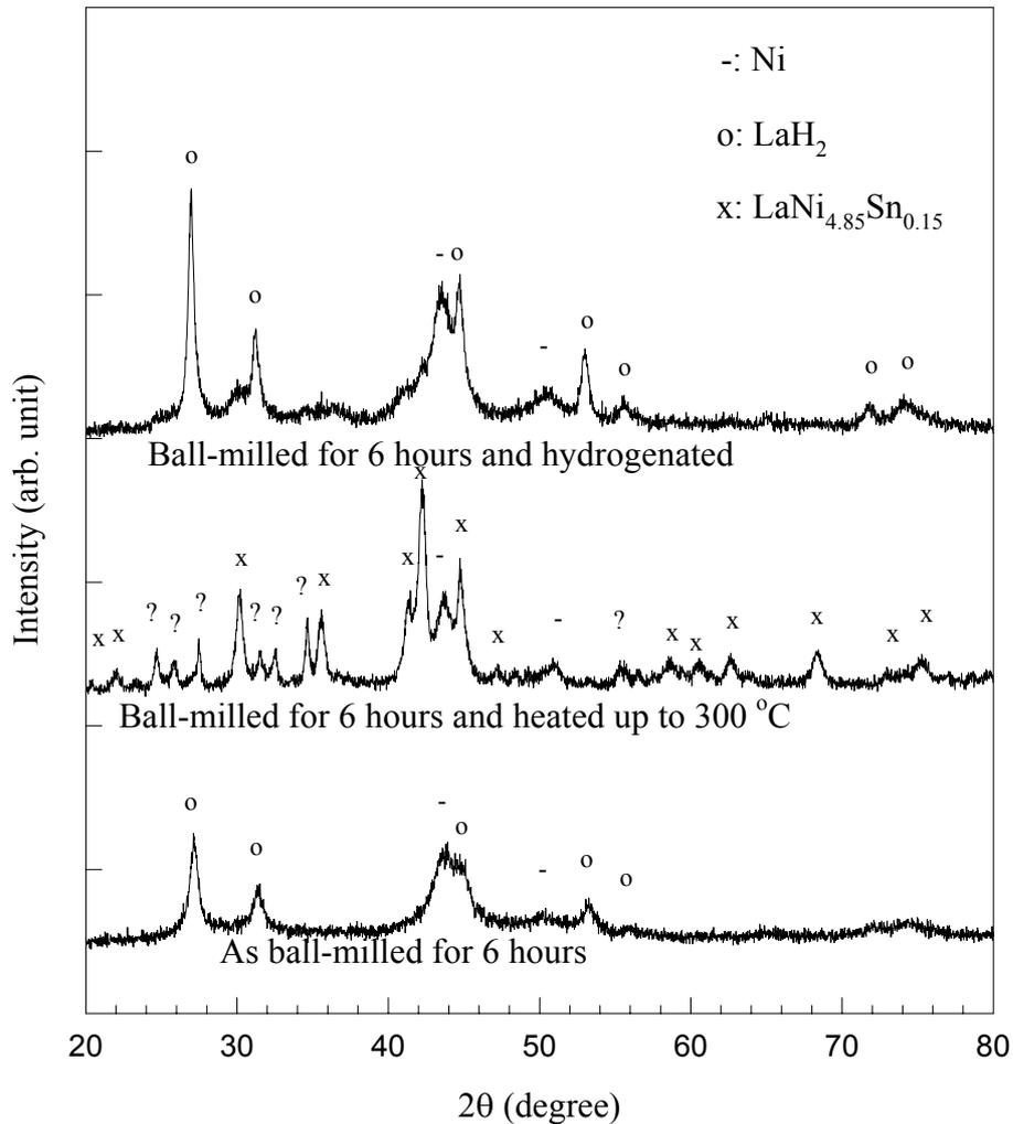
Figure 37. The XRD patterns of LiAlH<sub>4</sub> + LaNi<sub>4.85</sub>Sn<sub>0.15</sub> taken in 1:1 volume ratio and ball-milled for 6 hours, ball-milled for 6 hours and then heated to 300 °C for 15 min, and ball-milled for 6 hours, heated to 300 °C, and then hydrogenated.
