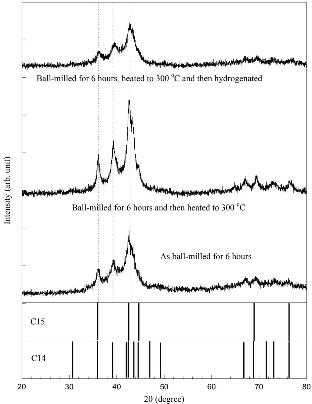
Figure 18. The XRD patterns of pure  $Zr_{27}Ti_9Ni_{38}V_5Mn_{16}Cr_5$  ball-milled for 6 hours, ball-milled for 6 hours and then heated to 300 °C for 15 min, and ball-milled for 6 hours, heated to 300 °C, and then hydrogenated.
