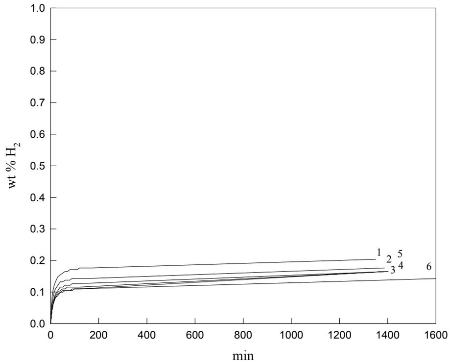
Figure 39. Hydrogenation behavior of pure  $\text{LaNi}_{4.85}\text{Sn}_{0.15}$  at 3.4-3.1 atm pressure at room temperature after ball-milling for 6 hours. The numeral next to the curve indicates hydrogenation cycle number.
