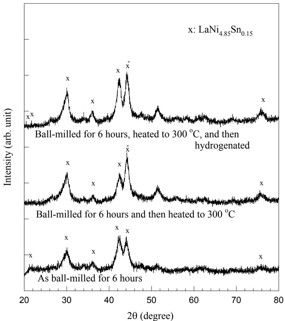
Figure 36. The XRD patterns of pure  $\text{LaNi}_{4.85}\text{Sn}_{0.15}$  ball-milled for 6 hours, ball-milled for 6 hours and then heated to 300 °C for 15 min, and ball-milled for 6 hours, heated to 300 °C, and then hydrogenated.
