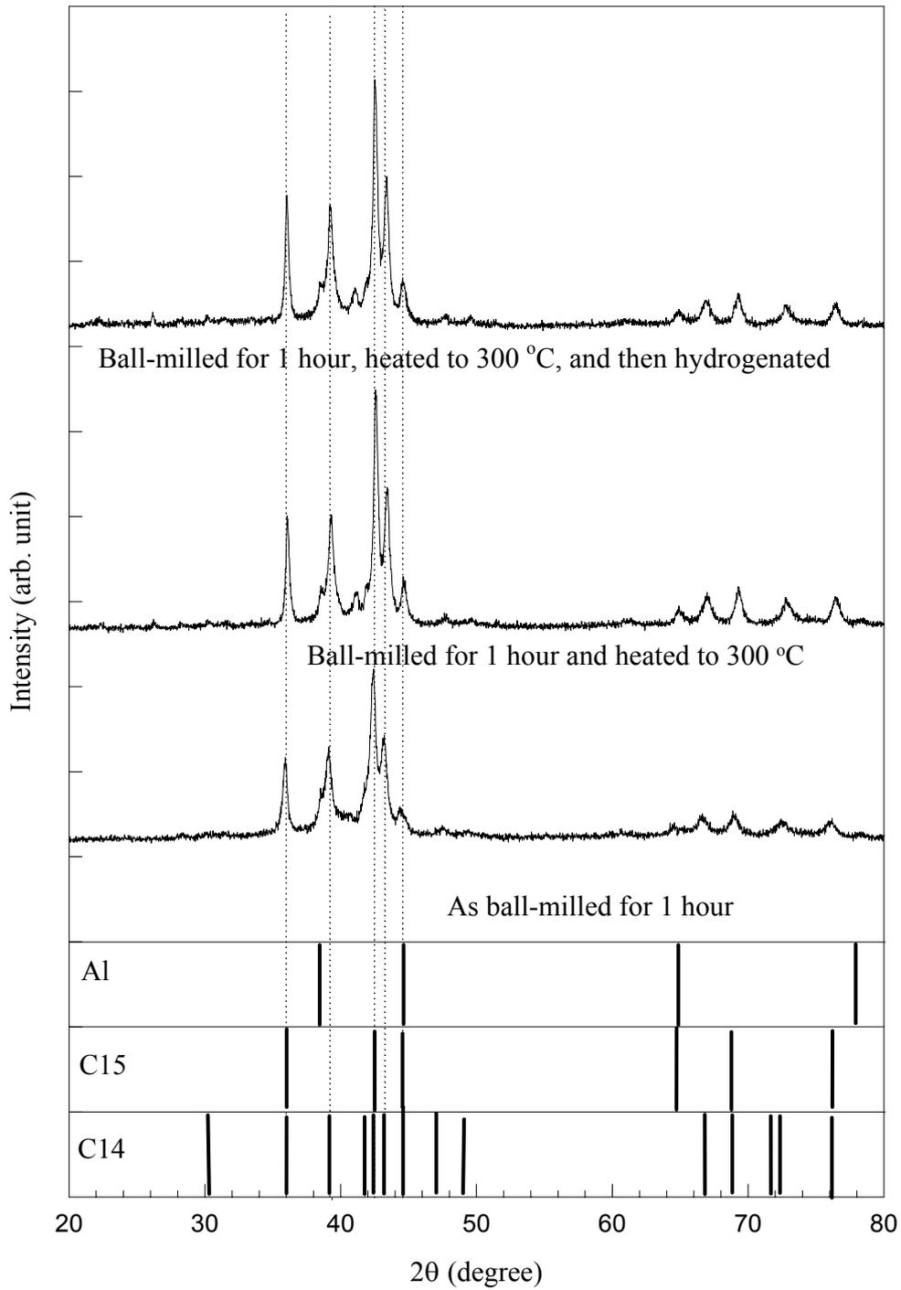
Figure 8. The XRD patterns of  $\text{LiAlH}_4 + \text{Zr}_{27}\text{Ti}_9\text{Ni}_{38}\text{V}_5\text{Mn}_{16}\text{Cr}_5$  taken in 1:1 volume ratio and ball-milled for 1 hour, ball-milled for 1 hour and then heated to 300 °C for 15 min, and ball-milled for 1 hour, heated to 300 °C, and then hydrogenated.
