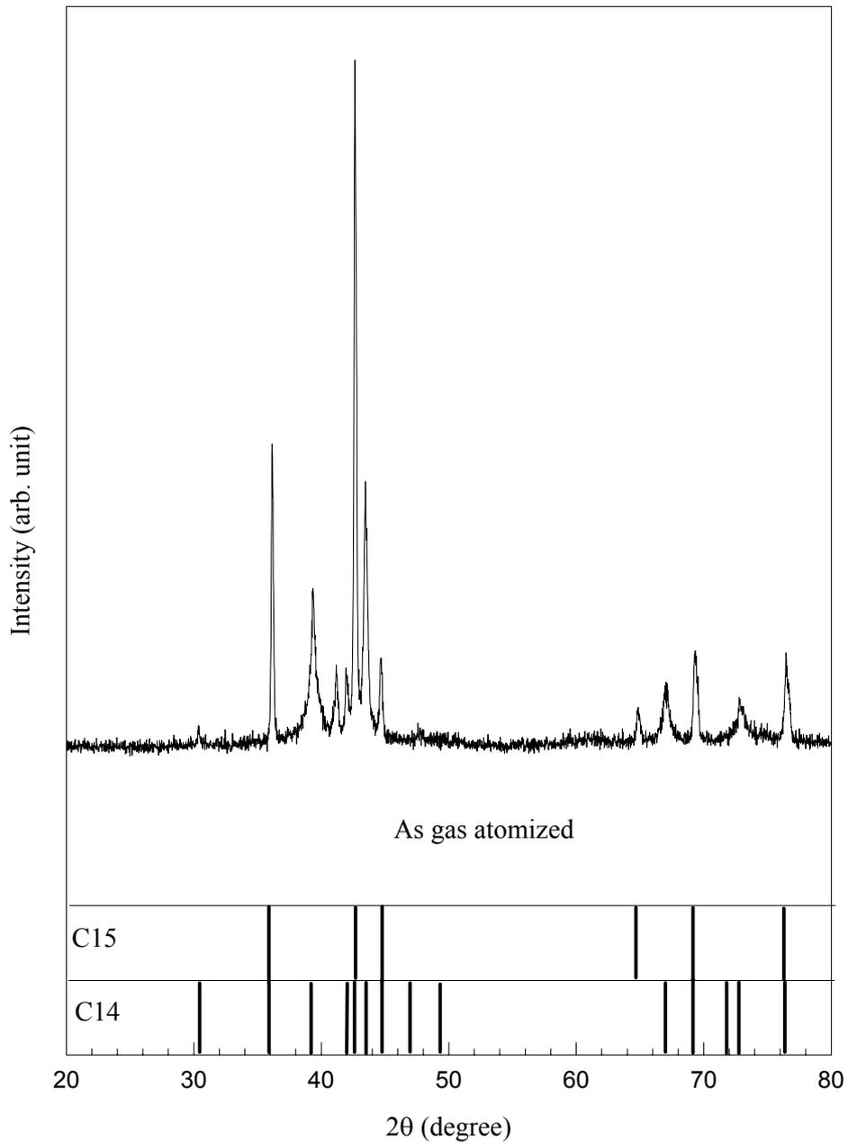
Figure 6. The XRD pattern of gas atomized  $Zr_{27}Ti_9Ni_{38}V_5Mn_{16}Cr_5$  powder. Vertical bars at the bottom indicate calculated Bragg peak positions of corresponding phases.
