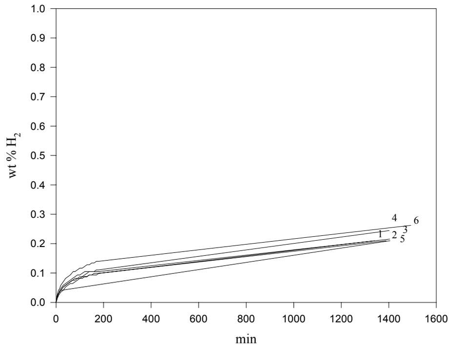
Figure 40. Hydrogenation behavior of  $\text{LiAlH}_4 + \text{LaNi}_{4.85}\text{Sn}_{0.15}$  at 3.4-3.1 atm pressure at room temperature taken in 1:1 volume ratio and ball-milled for 6 hours. The numeral next to the curve indicates hydrogenation cycle number.
