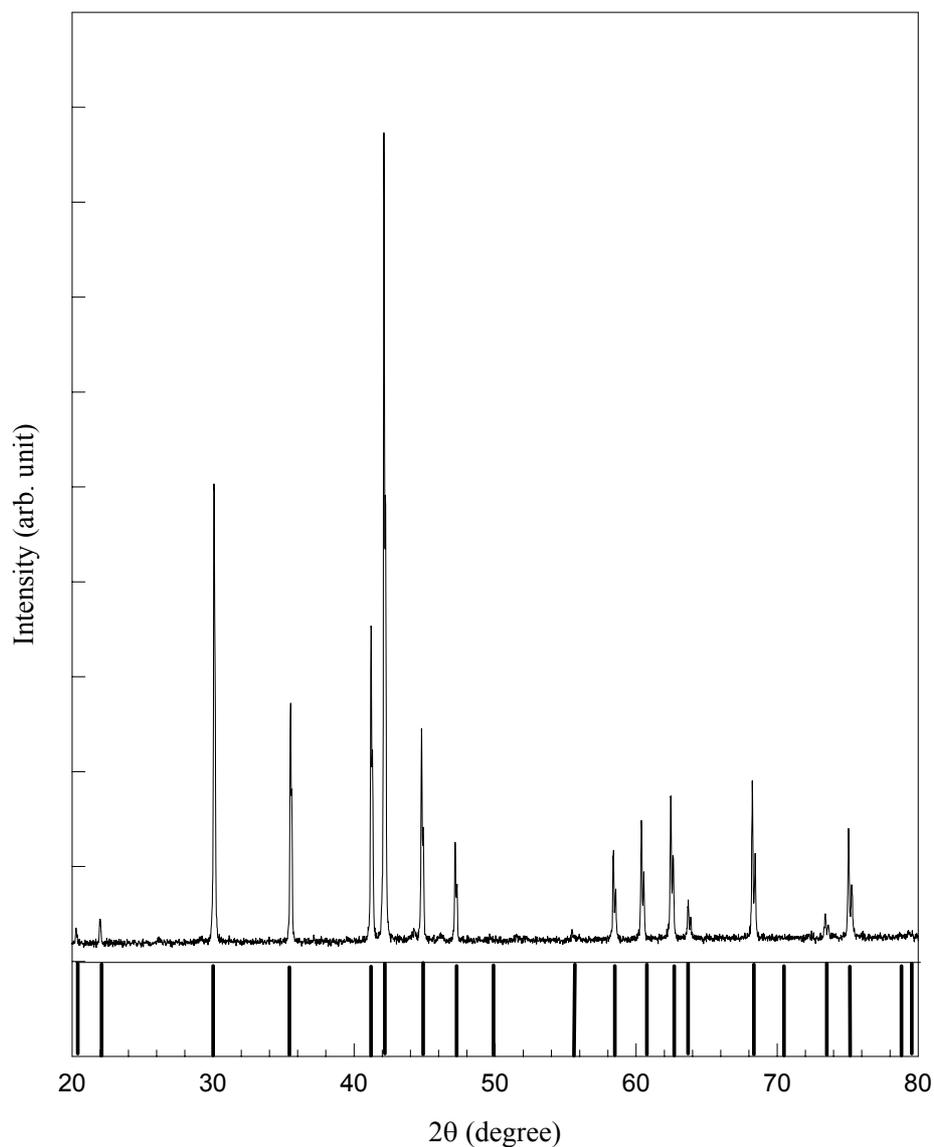
Figure 26. The XRD pattern of LaNi<sub>4.85</sub>Sn<sub>0.15</sub> annealed at 950 °C for 6 hours.
