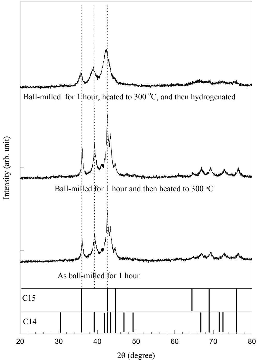
Figure 7. The XRD patterns of pure  $Zr_{27}Ti_9Ni_{38}V_5Mn_{16}Cr_5$  ball-milled for 1 hour, ball-milled for 1 hour and then heated to 300 °C for 15 min, and ball-milled for 1 hour, heated to 300 °C, and then hydrogenated.
