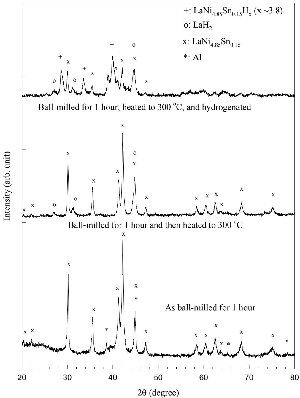
Figure 28. The XRD patterns of  $\text{LiAlH}_4 + \text{LaNi}_{4.85}\text{Sn}_{0.15}$  taken in 1:1 volume ratio and ball-milled for 1 hour, ball-milled for 1 hour and then heated to 300 °C for 15 min, and ball-milled for 1 hour, heated to 300 °C, and then hydrogenated.
