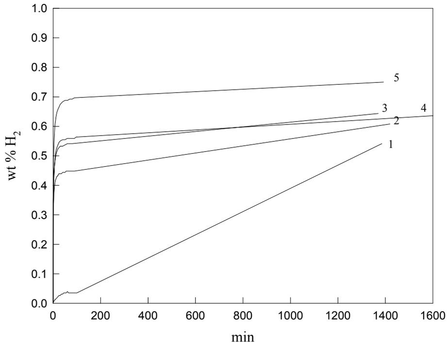
Figure 32. Hydrogenation behavior of  $\text{LiAlH}_4 + \text{LaNi}_{4.85}\text{Sn}_{0.15}$  at 3.3-2.2 atm pressure at room temperature taken in 1:1 volume ratio and ball-milled for 1 hour. The numeral next to the curve indicates hydrogenation cycle number.
