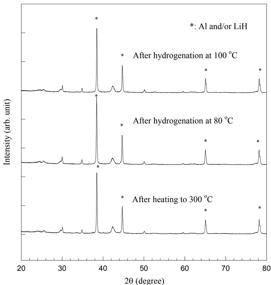
Figure 48. The XRD patterns of  $\text{LiAlH}_4 + 3 \text{ mol\% PdCl}_2$  ball-milled for 7 hours and then heated to  $300 \text{ }^\circ\text{C}$  for 15min, and ball-milled for 7 hours, heated to  $300 \text{ }^\circ\text{C}$ , and then hydrogenated at 68 atm pressure at 80 and  $100 \text{ }^\circ\text{C}$ .
