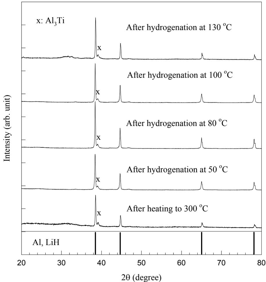
Figure 45. The XRD patterns of  $\text{LiAlH}_4 + 3 \text{ mol\% Al}_3\text{Ti}$  ball-milled for 7 hours and then heated to  $300 \text{ }^\circ\text{C}$  for 15min, and ball-milled for 7 hours, heated to  $300 \text{ }^\circ\text{C}$ , and then hydrogenated at 68 atm pressure at 50, 80, 100, and  $130 \text{ }^\circ\text{C}$ .
