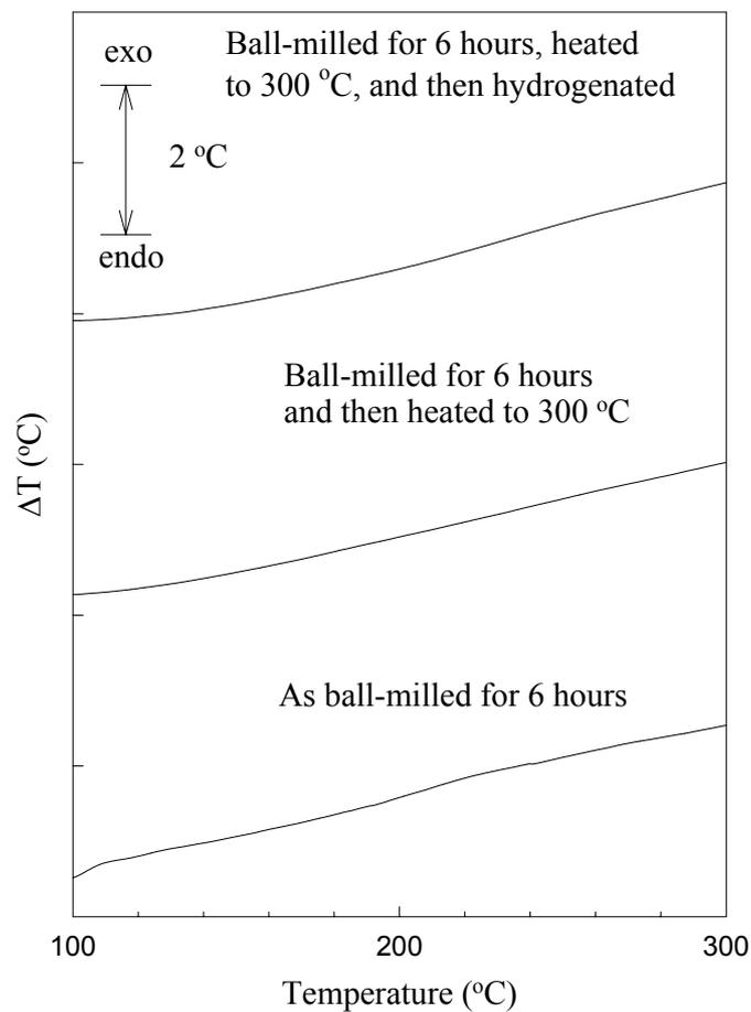
Figure 20. The DTA traces of pure  $\text{Zr}_{27}\text{Ti}_9\text{Ni}_{38}\text{V}_5\text{Mn}_{16}\text{Cr}_5$  ball-milled for 6 hours, ball-milled for 6 hours and then heated to 300 °C for 15 min, and ball-milled for 6 hours, heated to 300 °C, and then hydrogenated.
