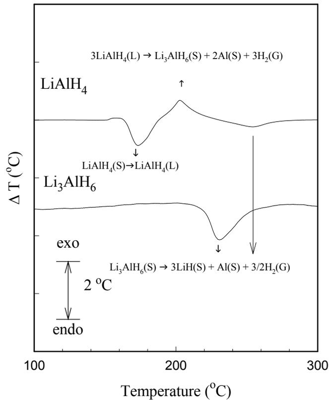
Figure 12. The DTA traces of  $\text{LiAlH}_4$  and  $\text{Li}_3\text{AlH}_6$  [21].
