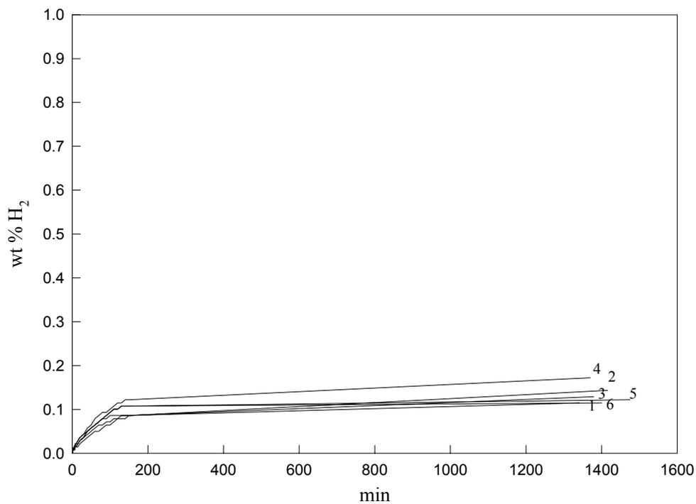
Figure 22. Hydrogenation behavior of pure  $Zr_{27}Ti_9Ni_{38}V_5Mn_{16}Cr_5$  at 3.4-3.2 atm pressure at room temperature after ball-milling for 6 hours. The numeral next to the curve indicates hydrogenation cycle number.
