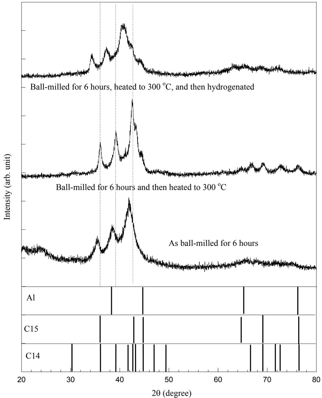
Figure 19. The XRD patterns of  $\text{LiAlH}_4 + \text{Zr}_{27}\text{Ti}_9\text{Ni}_{38}\text{V}_5\text{Mn}_{16}\text{Cr}_5$  taken in 1:1 volume ratio and ball-milled for 6 hours, ball-milled for 6 hours and then heated to 300 °C for 15 min, and ball-milled for 6 hours, heated to 300 °C, and then hydrogenated.
