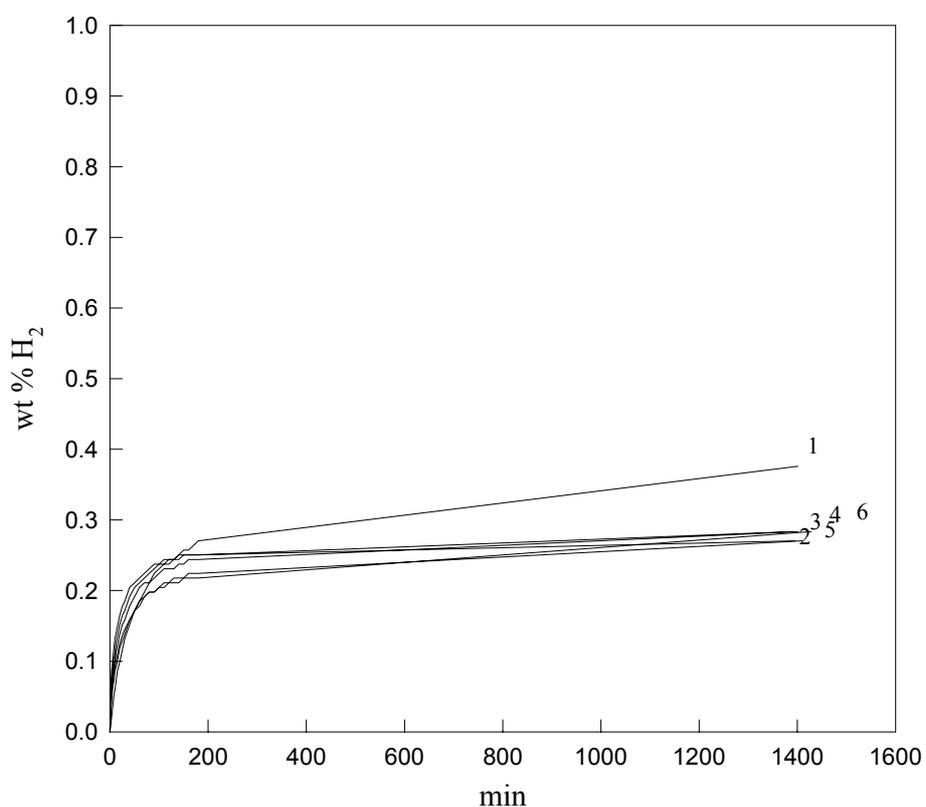
Figure 31. Hydrogenation behavior of pure  $\text{LaNi}_{4.85}\text{Sn}_{0.15}$  at 3.4-3.1 atm pressure at room temperature after ball-milling for 1 hour. The numeral next to the curve indicates hydrogenation cycle number.
