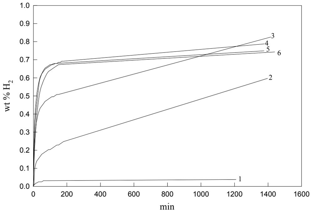
Figure 13. Hydrogenation behavior of pure  $Zr_{27}Ti_9Ni_{38}V_5Mn_{16}Cr_5$  at 3.4-2.5 atm pressure at room temperature after ball-milling for 1 hour. The numeral next to the curve indicates hydrogenation cycle number.
