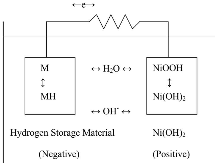
Figure 3. A schematic of the secondary battery with hydrogen storage materials.
