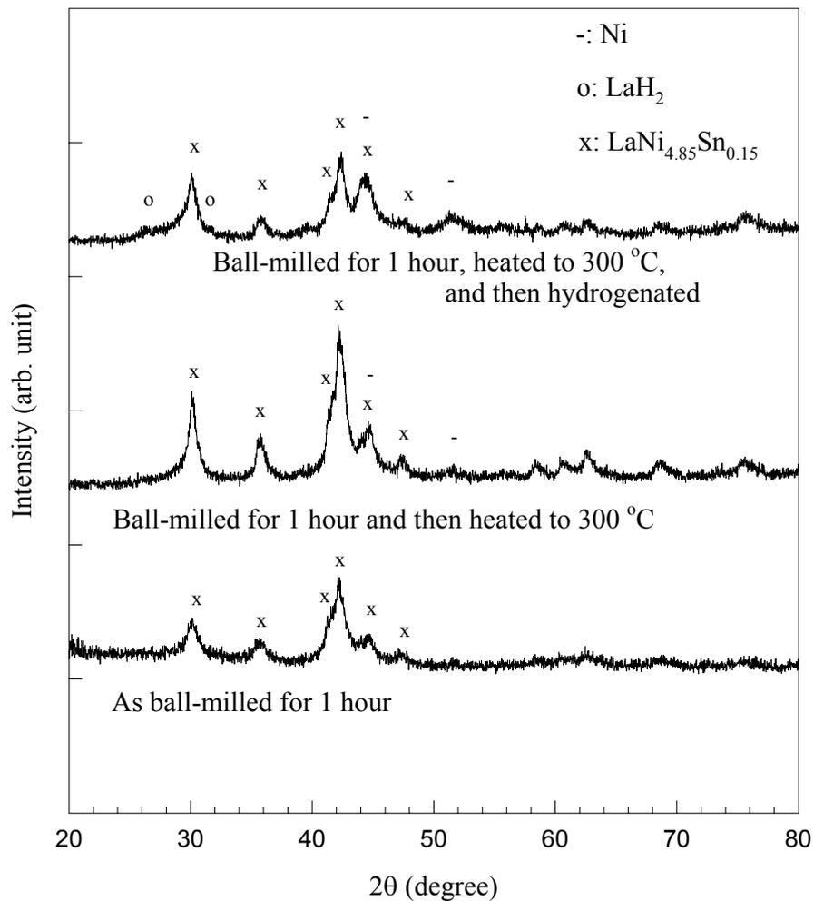
Figure 27. The XRD patterns of pure  $\text{LaNi}_{4.85}\text{Sn}_{0.15}$  ball-milled for 1 hour, ball-milled for 1 hour and then heated to 300 °C for 15 min, and ball-milled for 1 hour, heated to 300 °C, and then hydrogenated.
