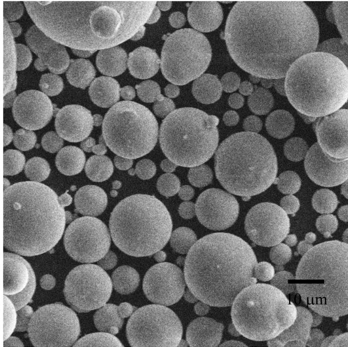
Figure 15. Morphology of gas atomized  $Zr_{27}Ti_9Ni_{38}V_5Mn_{16}Cr_5$  (x 1000).
