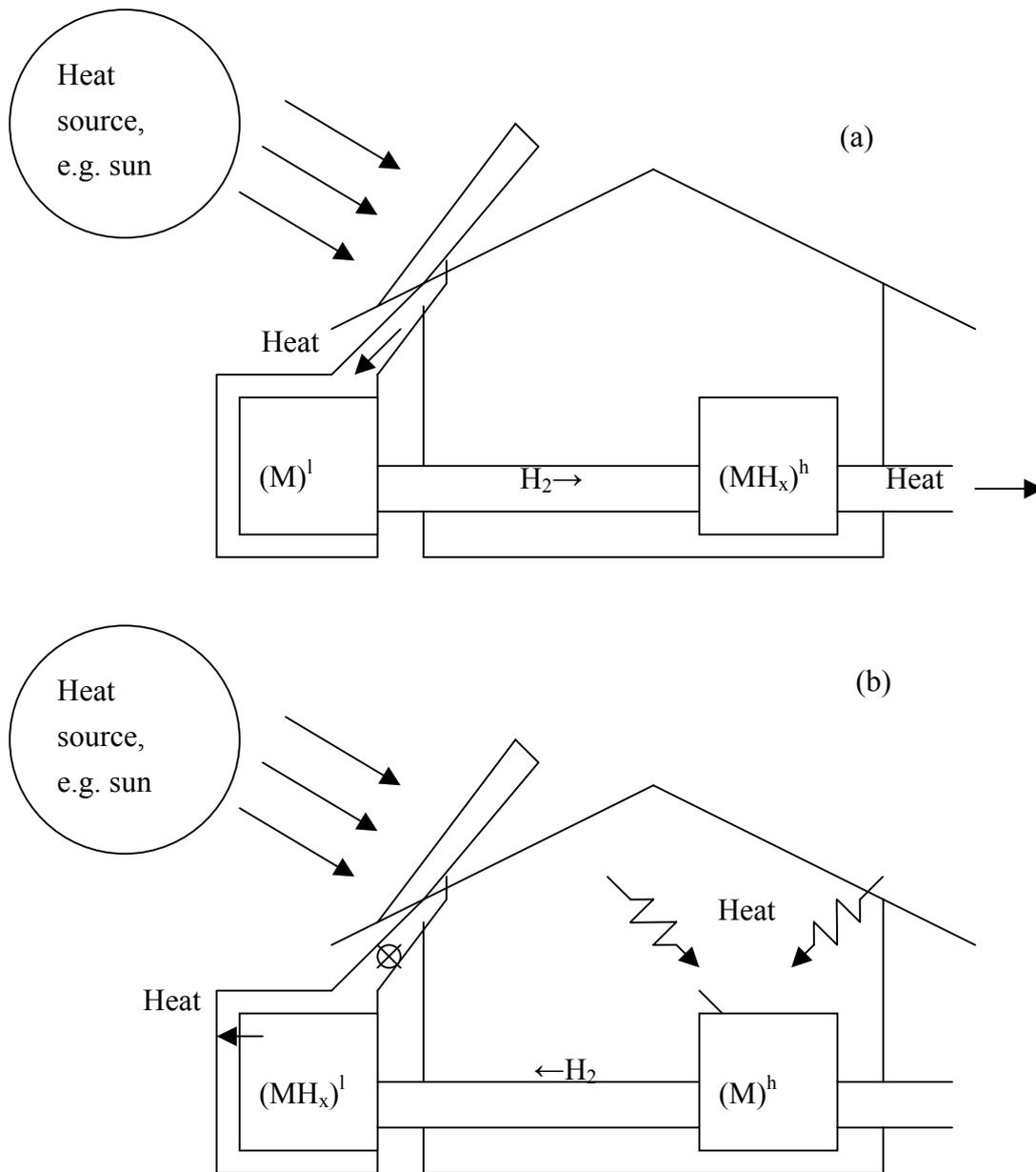
Figure 2. The principle of the cooling system using two solid state hydrides with different equilibrium hydrogen pressure.  $(MH_x)^l$ - hydride with low equilibrium pressure,  $(MH_x)^h$ - hydride with high equilibrium pressure.
