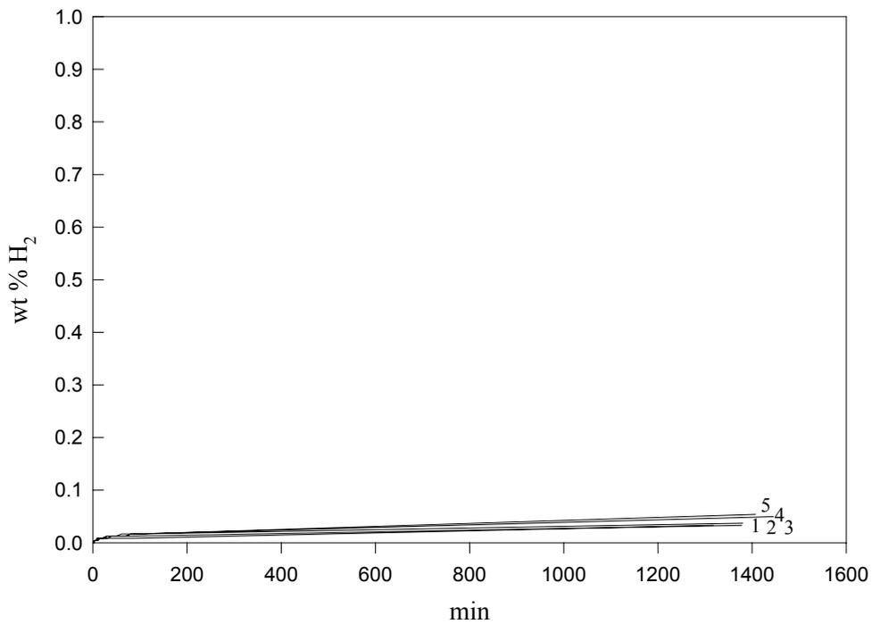
Figure 14. Hydrogenation behavior of  $LiAlH_4 + Zr_{27}Ti_9Ni_{38}V_5Mn_{16}Cr_5$  at 3.4-3.3 atm pressure at room temperature taken in 1:1 volume ratio and ball-milled for 1 hour. The numeral next to the curve indicates hydrogenation cycle number.
