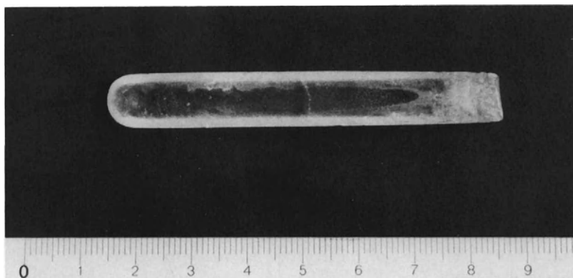
Fig. 11. \text{RbMnF}_3 crystal (melting-zone technique). Scale in centimeters.
