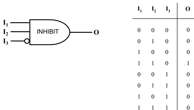
Fig. 13: An INHIBIT gate with its corresponding truth table.
