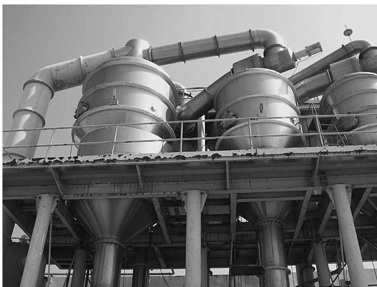
Figure 7.12 Typical evaporator unit.
