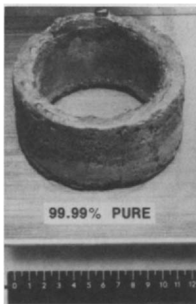
FIG. 10. 5.3 kg of ultrapure (99.99% by wt) Pu metal produced by electrorefining in a molten salt.
