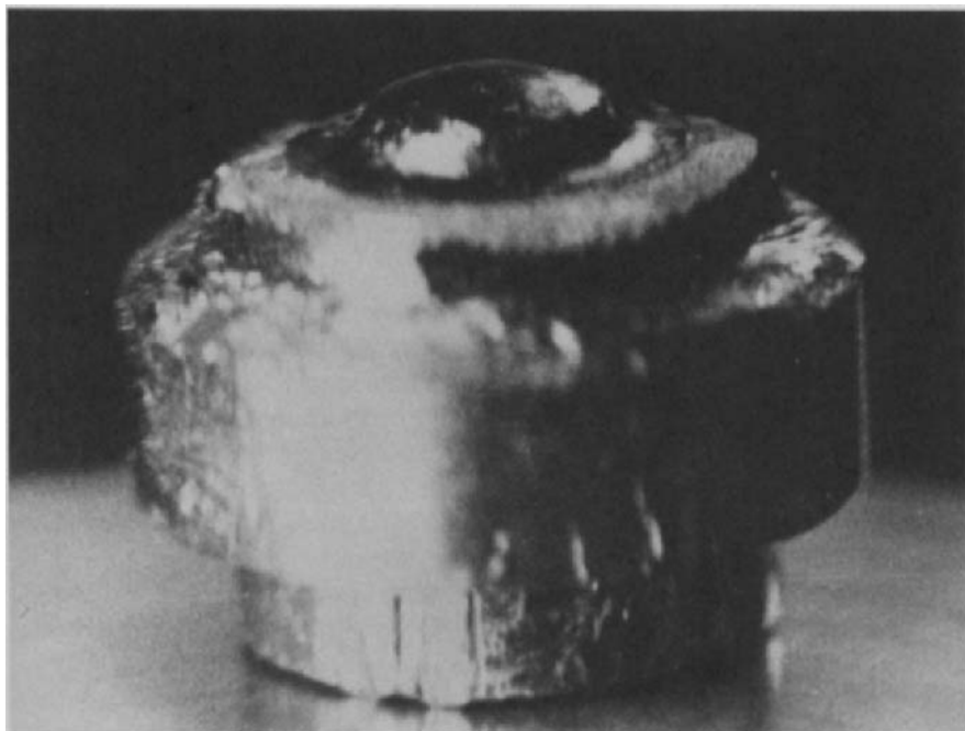
FIG. 13. A mass of Cm metal produced by distillation and deposition in a Ta still.
