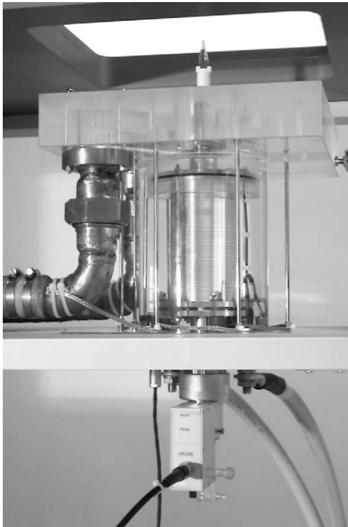
FIG. 8. The 1 T magnet assembled inside its enclosure.
