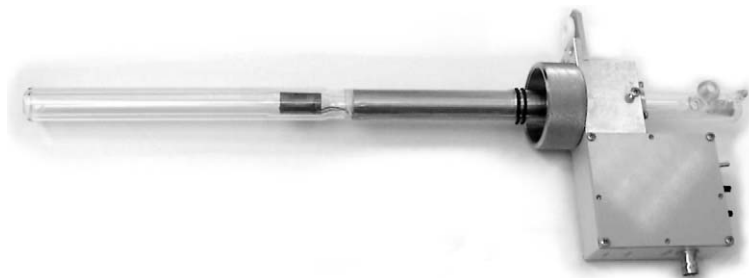
FIG. 18. A FFC signal detection probe.
