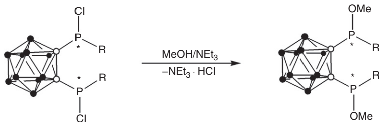
FIG. 5. Illustration of the inhibited methanolysis of P – Cl bounds observed for ortho -carborane (12) derivatives.
