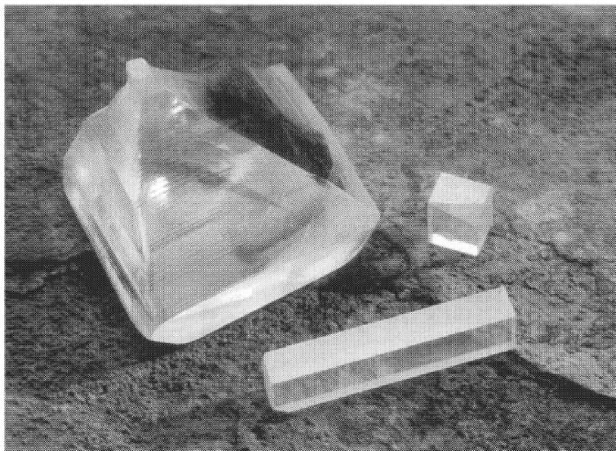
Figure 1. As-grown crystal of potassium niobate with two optical elements cut from similar top-seeded crystals. (Courtesy of P. Bordui, Crystal Technology.)
