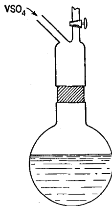
FIG. 11. Apparatus for the preparation of vanadium(II) hydroxide.
