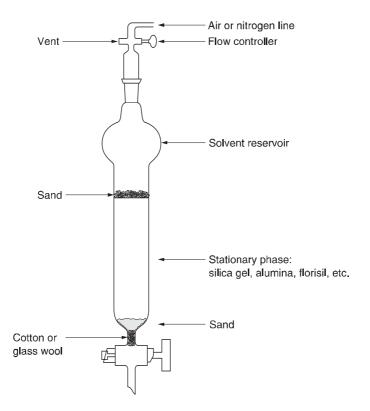
Figure 1.5 Typical flash chromatography setup.
