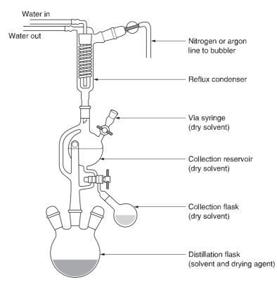
Figure 1.1 Solvent distillation setup.
