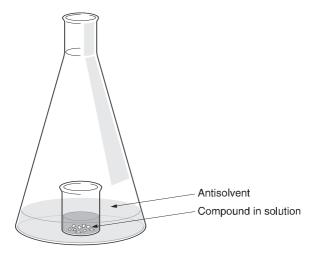
Figure 1.7 Crystallization setup.
