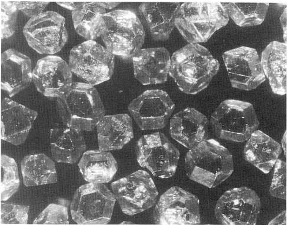
Figure 12.6. Typical high-pressure synthetic diamond crystals. .(Photograph courtesy of GE Superabrasives, Worthington, OH.)
