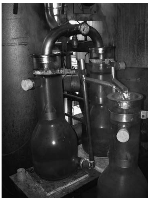
FIGURE 4.19 Orris distillation, Florentine flask at nearly 98°C.
