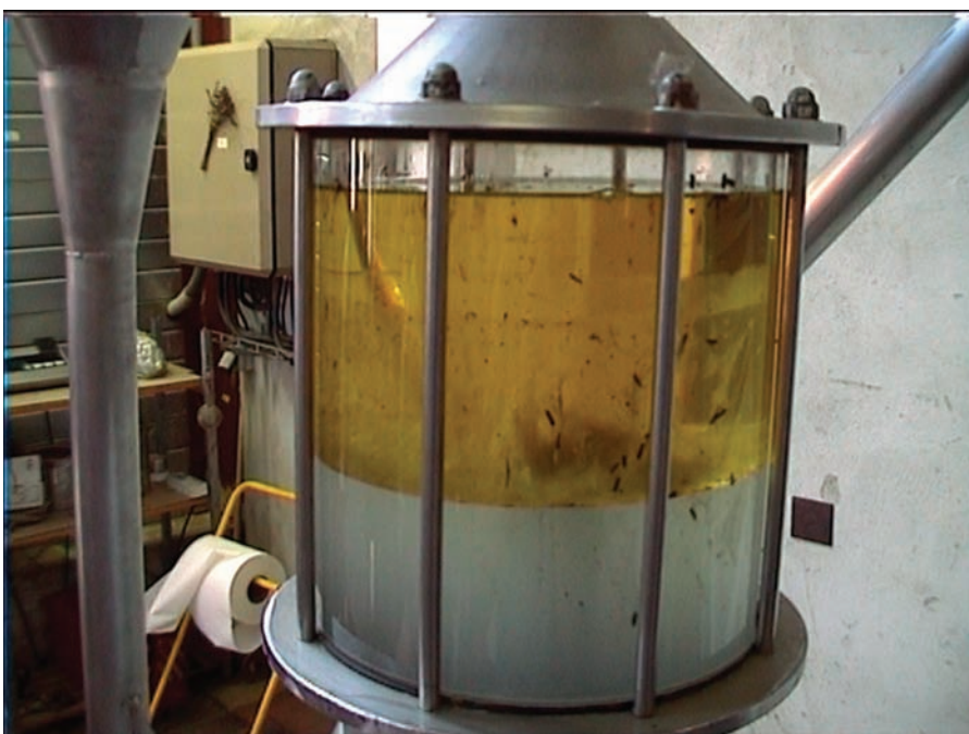
FIGURE 4.18 Oil and muddy water in the Florentine flask.
