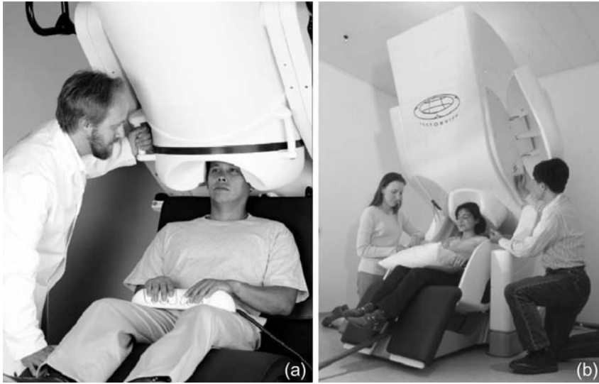
Fig. 11.8 Whole-cortex MEG instrumentation of 4D Neuroimaging [10] and Elekta Neuromag Oy [9] for seated or supine subjects: (a) Magnes 2500WH or Magnes 3600WH (courtesy of 4D Neuroimaging Inc.); (b) Elekta Neuromag® (courtesy of Elekta Neuromag Oy).
