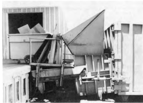
FIG. 25-60 Small compactor used in conjunction with a detachable roll-off container. Note the wheeled container used to collect wastes within the warehouse.
