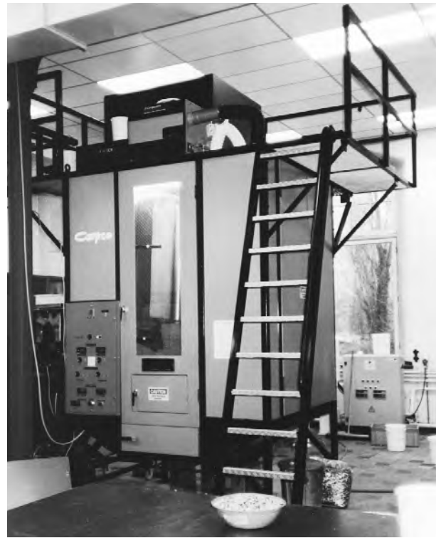
FIG. 19-62 New Triboelectric separator for separation of PVC from other plastics. (Courtesy Carpco, Inc.)
