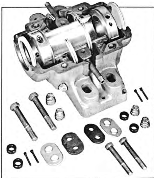
FIG. 29-63 Typical oil-film pillow-block bearing. Lubrication is provided both by an oil flow and by oil rings.
