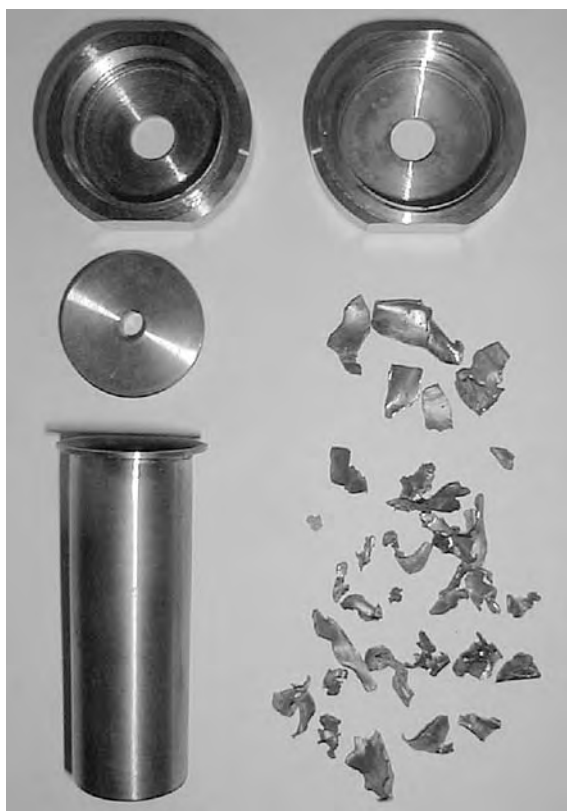
Fig. 33 Steel sleeve test of DNB (10 g, 6 mm) before ( left ) and after test ( right )
