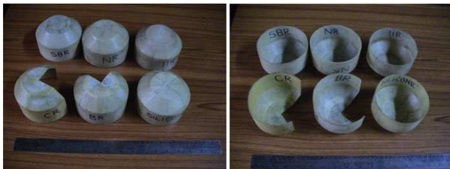
Fig. 3.9 FRP components made by RPM [1–4]
