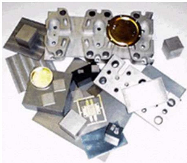
Fig. 11.26 Discontinuously reinforced Al MMCs for electronic packaging applications: cast graphite–Al composite components [1]
