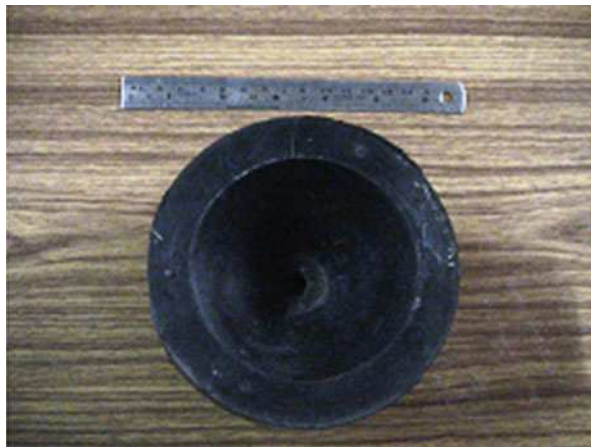
Fig. 3.6 Photograph of rubber punch [1–4]
