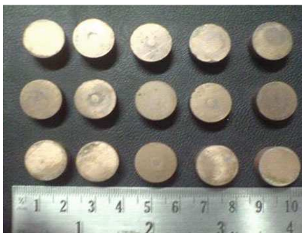
Fig. 13.4 Typical copper–graphite composite processed through P/M route
