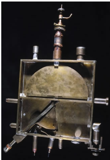
Figure 1. Cyclotron built by E. Lawrence and S. Livingston in 1931. (from the National Museum of Science and Industry, UK)
