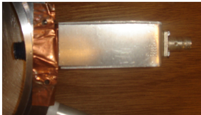
Figure 13. Proton detector and copper flashing which ensures constant connection to ground and shields detector.
