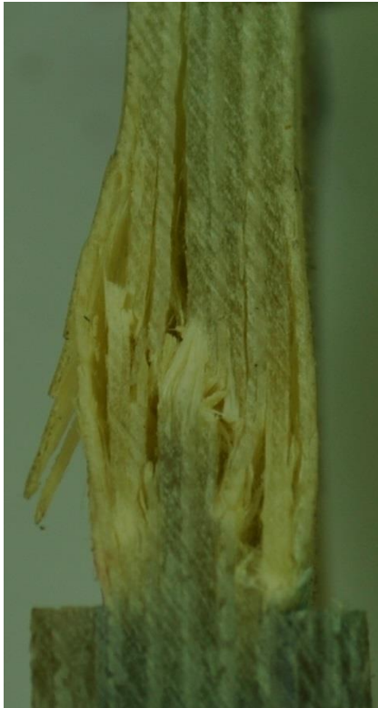
Figure 28: Buckling of plies and secondary delamination
