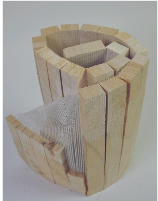
Figure 16: Core material with grooves (source: WMC)
