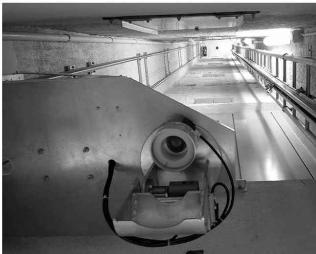
Fig. 4. The drop-tower seen from below. The system consists essentially of a vertical shaft in which a steel ball can be moved to a certain height and then dropped onto the test-object.
