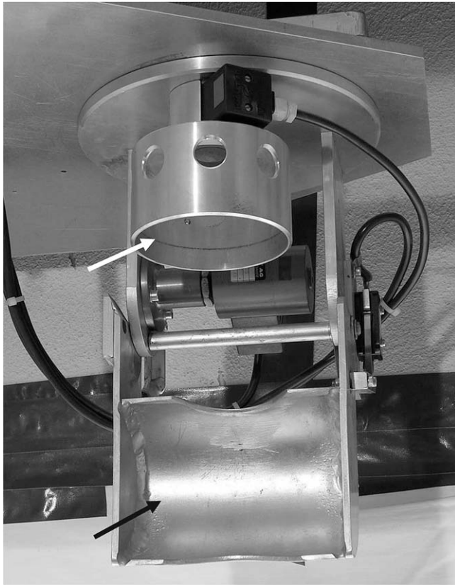
Fig. 5. The releasing mechanism of the drop-tower. A steel trap (black arrow) secures the ball until the ball is to be dropped. After releasing this safety-trap, the ball is still fixed onto a magnetic ring (white arrow). The magnetic field can then be interrupted, causing the ball to fall.
