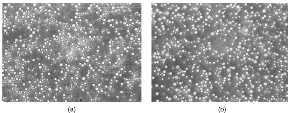
**Figure 15.6** Optical micrographs of O/W emulsions stabilized with HMI stored at 50 °C for (a) 1.5 weeks and (b) 14 weeks.
