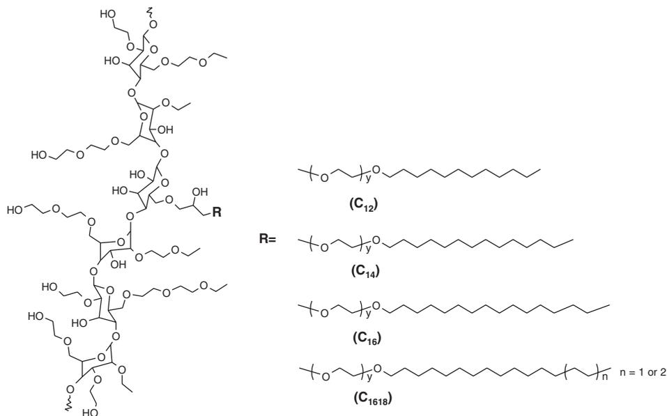
**Figure 13.3** Possible structure segment of the HM-EHECs studied in Reference [12].  $R = (C_{12})$  for HM-( $C_{12}$ )-EHEC,  $R = (C_{14})$  for HM-( $C_{14}$ )-EHEC,  $R = (C_{16})$  for HM-( $C_{16}$ )-EHEC and  $R$  is a blend of ( $C_{16}$ ) and ( $C_{18}$ ) for HM-( $C_{16,18}$ )-EHEC.
