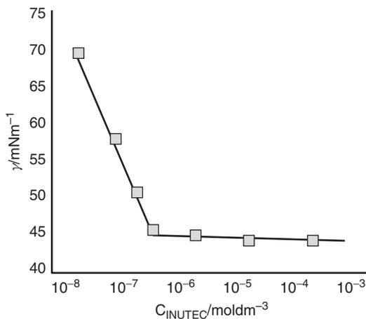
Figure 15.3  $\gamma - \log C_{HMI}$  curve at the air/water interface.
