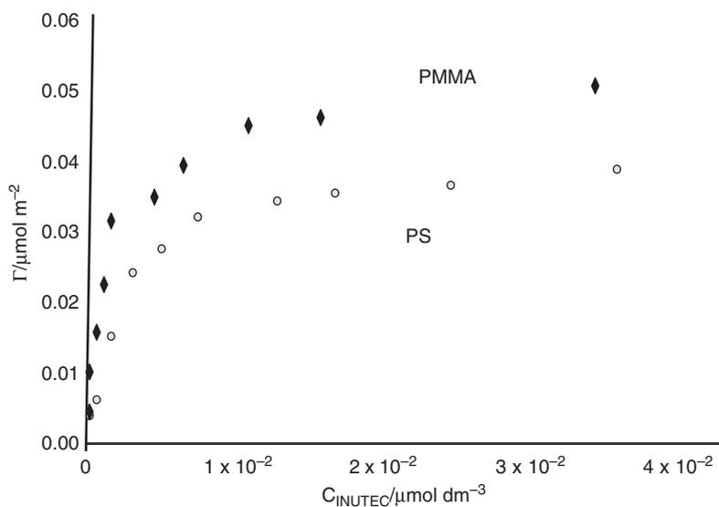
**Figure 15.5** Adsorption isotherms of HMI on PS and PMMA latexes.
