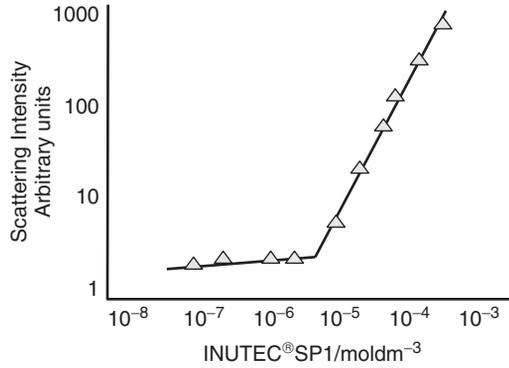
Figure 15.2 Light scattering intensity as a function of HMI concentration.
