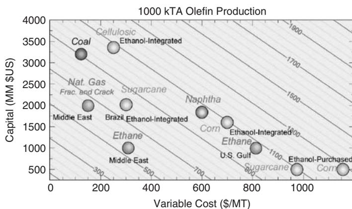
**Figure 6.3** Contour plot of production cost plus return of investment as a function of capital and variable costs (based on 1000 kilotonnes/year of olefin production). Diagonals = cost of production, MM \$US = million US dollars.
