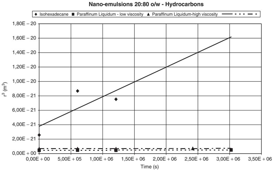
**Figure 15.14**  $r^3$  versus  $t$  for nanoemulsions based on hydrocarbon oils.
