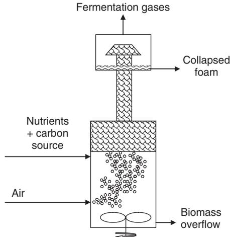
**Figure 9.5** Schematic of a continuous/batch fermenter with a foam fractionation unit.
