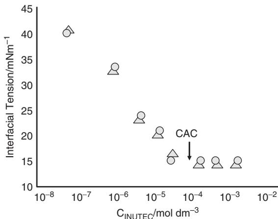
**Figure 15.4**  $\gamma - \log C_{\text{HMI}}$  curve at the oil/water interface;  $\Delta$ ,  $2 \times 10^{-4} \text{ mol/dm}^3$  NaCl;  $\circ$ ,  $5 \times 10^{-1} \text{ mol/dm}^3$  NaCl.
