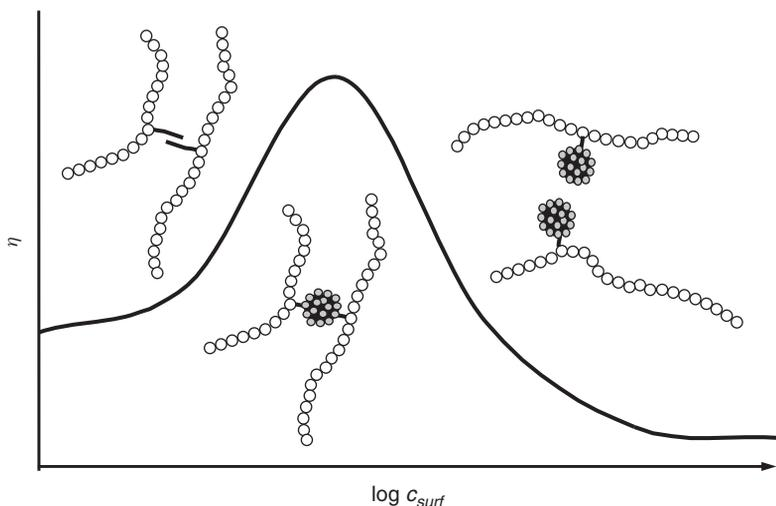
**Figure 13.9** Schematic illustration of the influence of surfactant concentration on the viscosity of solutions of HM polymers.
