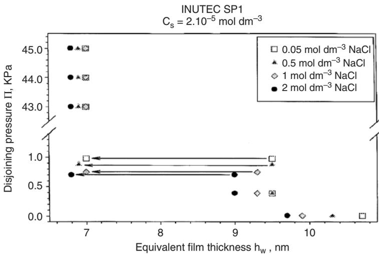
Figure 15.7 Variation of disjoining pressure with equivalent film thickness at various NaCl concentrations.
