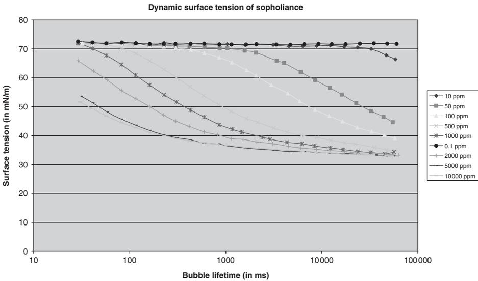
Figure 11.15 Dynamic surface tension (mN/m) of sophorolipids as a function of concentration and bubble lifetime.
