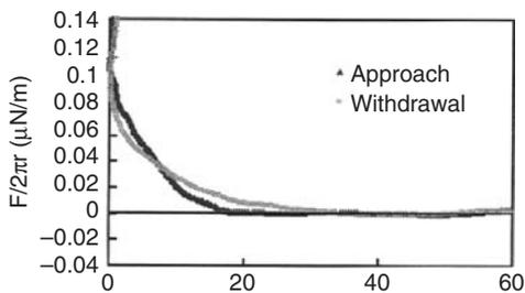
Figure 15.10 Force–distance (in nm) curves between hydrophobized glass surfaces containing adsorbed HMI in water.
