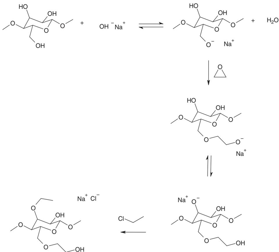
**Figure 13.1** The reaction scheme for production of ethyl hydroxyethyl cellulose (EHEC), which includes the reaction steps alkalization, ethoxylation and alkylation with ethyl chloride.
