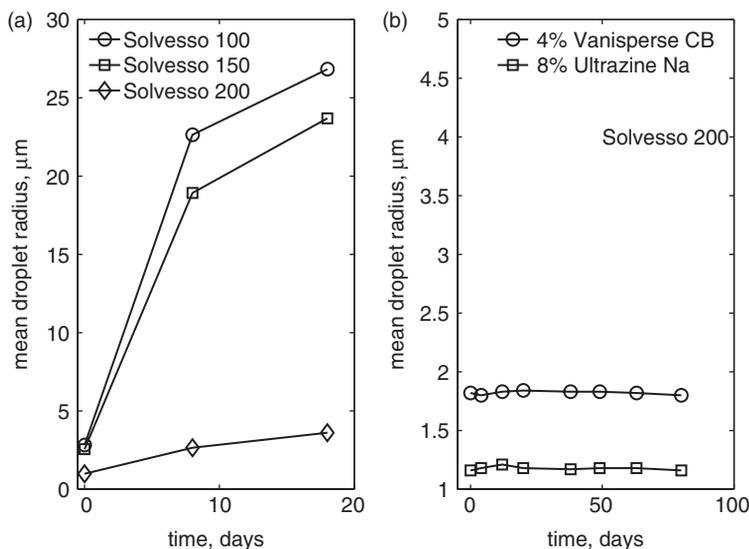
**Figure 14.5** (a) The increase in average droplet radius as a function of time of storage at 40 °C. Ostwald ripening takes place at different rates in the three systems. In (b) the average droplet radius is followed for 80 days without significant variation. In this system, 6% of a nonmobile component is added to the oil (Solvesso 200) and this effectively inhibits Ostwald ripening.
