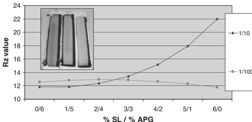
Figure 11.19 Cleaning efficiency as measured by the Rz value for sophorolipid and APG mixtures.
