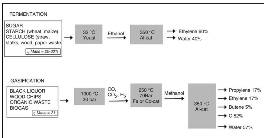
**Figure 6.1** Schematic process of fermentation and gasification routes for ethylene production from renewable feedstock.
