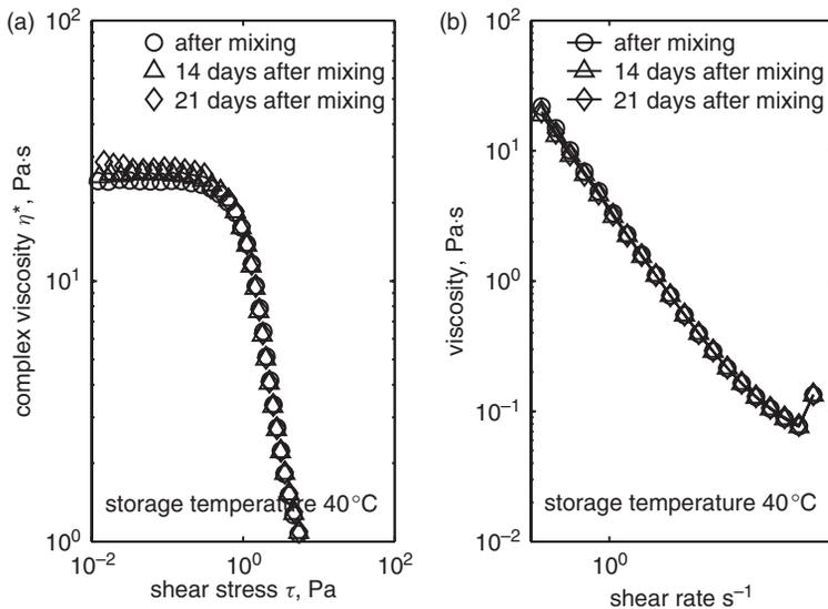
**Figure 14.7** (a) Amplitude sweeps and (b) flow curves of a suspoemulsion comprised of 23% sunflower oil, 23% Chlorothalonil, 4% lignosulfonate and biocide, wetting agent and xanthan gum for stabilizaton. The plateau value of the complex viscosity increases slightly with time, but the yield stress remains similar for the duration of the trial. From measurements of the shear viscosity, no changes are discerned in the flow curves (b).
