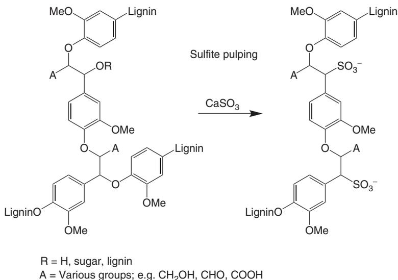
**Figure 14.2** A tentative description of the sulfite pulping process. Lignin in the structure represents the sites where the lignin structure propagates.
