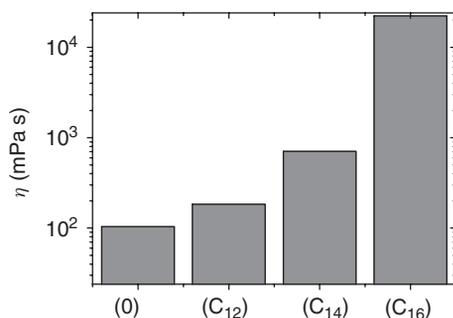
**Figure 13.6** Zero shear viscosity ( $\eta$ ) of 1% w/w solutions of HM-EHEC with varying lengths of the hydrophobic groups, where (0) represents unmodified EHEC.
