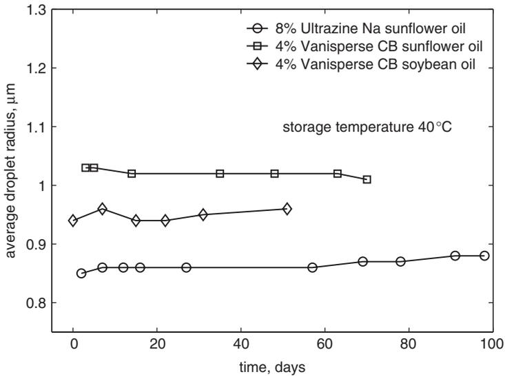
**Figure 14.6** Lignosulfonates stabilize vegetable oil emulsions, here demonstrated with soya bean oil and sunflower oil. No viscosity modifier was added so a creaming layer formed upon storage. Before measurement of the droplet size the emulsions were gently stirred for homogenization. No coalescence or flocculation was observed and the droplet size remained constant.
