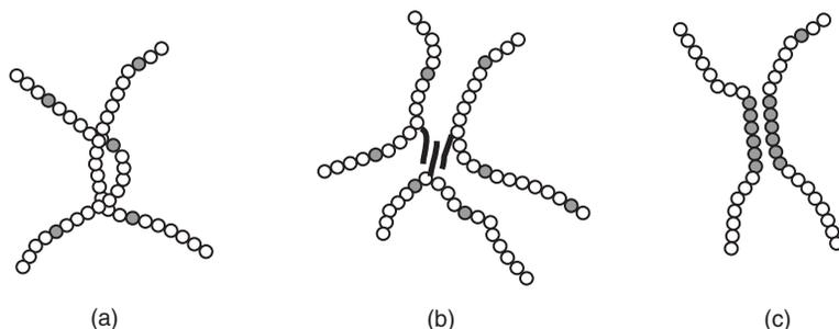
**Figure 13.4** Schematic illustrations of the different types of interpolymeric cross-links in HM-EHEC solution: (a) chain entanglements, (b) associations between hydrophobic side chains and (c) associations between hydrophobic segments of the polymer backbone. Unfilled rings represent hydrophilic glucose units, filled rings represent hydrophobic glucose units and bold lines represent hydrophobic side chains.
