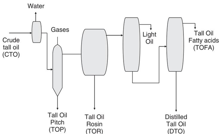
**Figure 3.2** *Principal scheme and main products of crude tall oil distillation.*
