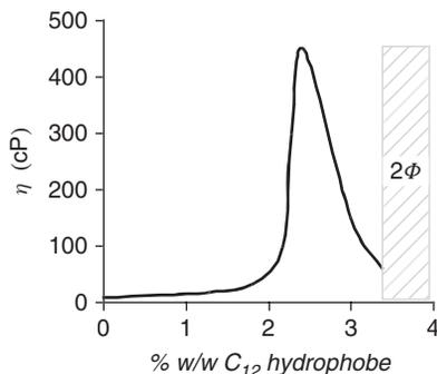
**Figure 13.7** Brookfield viscosity of 2% w/w solution of HM-HEC substituted with 1,2-epoxydodecane as a function of degree of hydrophobic modification.
