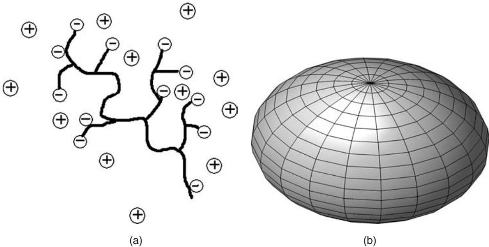
**Figure 14.1** A schematic figure illustrating a possible lignosulfonate structure. The longest chain fragment constitutes a lignosulfonate backbone and shorter chains are grafted to this backbone (a). According to Vainio *et al.* [5], the shape of a lignosulfonate molecule can be approximated by an ellipsoid (b), as shown to the right. The two representations are not to scale.
