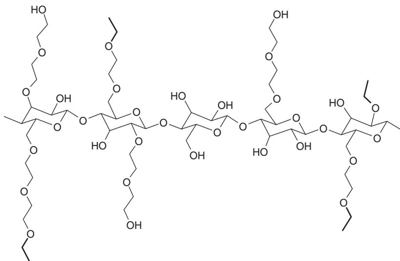
**Figure 13.2** Possible structure element of an EHEC molecule, where  $\text{---}\text{O}$  represents a hydroxyethyl group and ethyl groups are represented by bold lines. In this example  $MS_{EO} = (4 + 3 + 0 + 2 + 1)/5 = 2$  and  $DS_{ethyl} = (1 + 1 + 0 + 0 + 2)/5 = 0.8$ .
