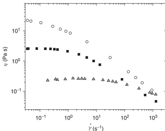
**Figure 13.8** Viscosity ( $\eta$ ) as a function of shear rate ( $\dot{\gamma}$ ) for solutions of high MW EHEC 1% in water ( $\circ$ ), low MW EHEC 2% in water ( $\blacktriangle$ ) and HM-EHEC 1% in water ( $\blacksquare$ ).
