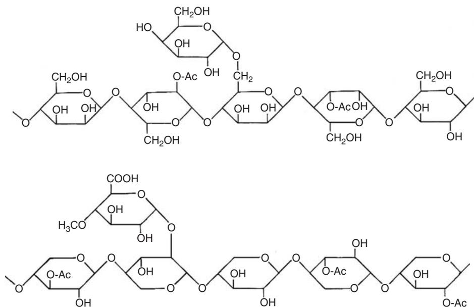
**Figure 3.8** Principal structure of the main softwood hemicellulose type, galactoglucomannan, and of the main hardwood hemicellulose type, 4-O-methyl glucuronoxylan.
