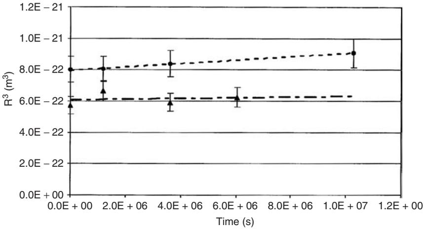
**Figure 15.13** Silicone oil in water nanoemulsions stabilized with HMI (top curve: 1.6% w/w HMI; bottom curve: 2.4% w/w HMI).
