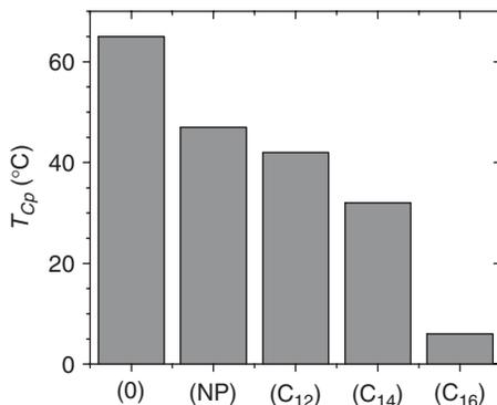
**Figure 13.10**  $T_{Cp}$  of 1% w/w solutions of HM-EHEC with varying lengths of the hydrophobic groups, where (0) represents unmodified EHEC.
