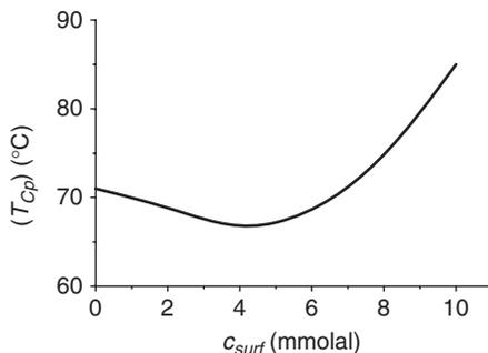
**Figure 13.11**  $T_{Cp}$  as a function of sodium dodecyl sulfate concentration for 0.9% w/w solution of EHEC. Reproduced from *J. Phys. Chem.*, 1990, **94** (12), 5005–5015.
