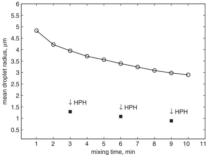
**Figure 14.4** The circles describe the reduction in average droplet radius as a function of mixing time in a high-shear mixer. At three times during high-shear mixing, a pre-emulsion may be further homogenized in a high-pressure homogenizer, which reduces the average droplet radius further (squares). In this example the emulsion is composed of equal parts of water and soya bean oil and 4 mass % lignosulfonate as stabilizer.
