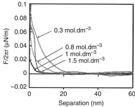
**Figure 15.11** Force–distance curves for hydrophobized glass surfaces containing adsorbed HMI at various  $\text{Na}_2\text{SO}_4$  concentrations.
