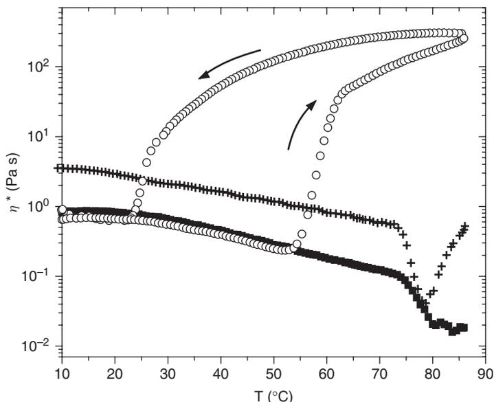
**Figure 13.12** Complex viscosity ( $\eta^*$ ) as a function of temperature for 1% w/w polymer solutions of (+) Bermocoll E481FQ (EHEC), (○) Methocel A16M (MC) and (■) Methocel K15M (HPMC). The heating and cooling rates are  $1.5^\circ/\text{min}$ .
