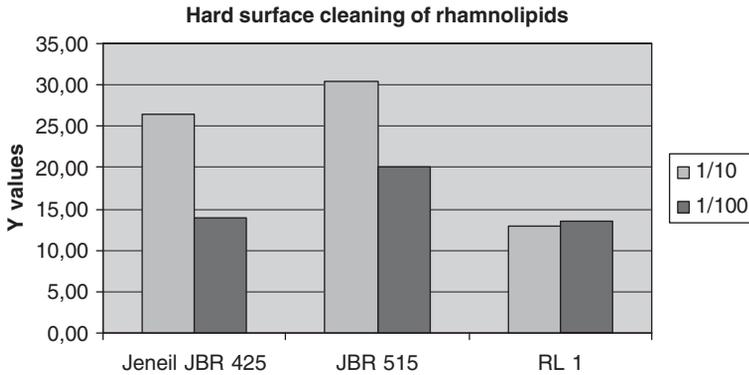
**Figure 11.17** Hard surface cleaning performance of JBR425, JBR515 and RL1 (Stuttgart) in concentrated and diluted applications.
