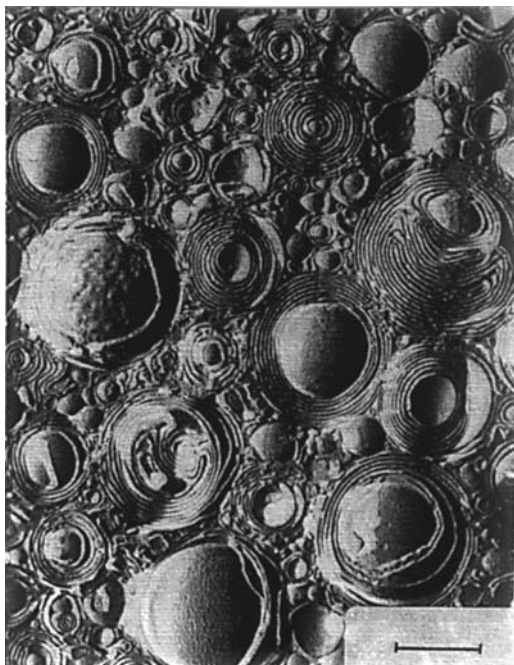
Figure 1.9 Freeze-fracture electron micrograph showing the onion phase of vesicles present in the tetradecyldimethylamineoxide/hexanol/water system (bar = 1 \mu\text{m} ). Reproduced from reference 58 with permission of Academic Press/Elsevier.
