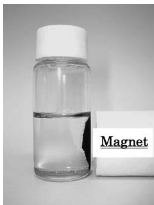
Figure 5.4 Separation of the RuHAP- \gamma -Fe 2 O 3 catalyst from a reaction mixture by application of an external permanent magnet.
