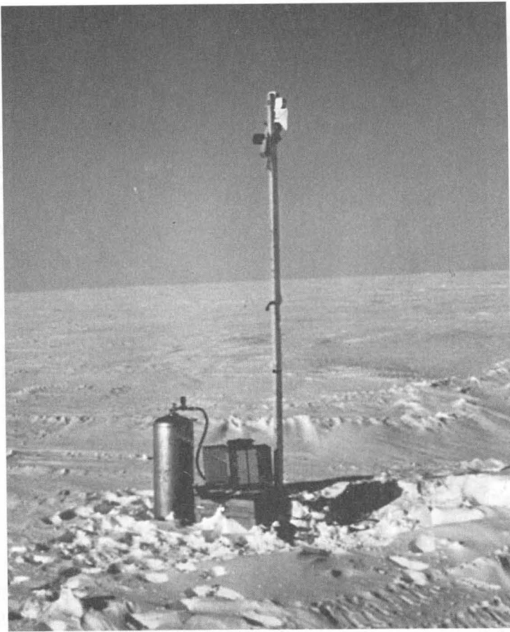
FIGURE 6 TEG-powered radionavigation transponder, Canada.
