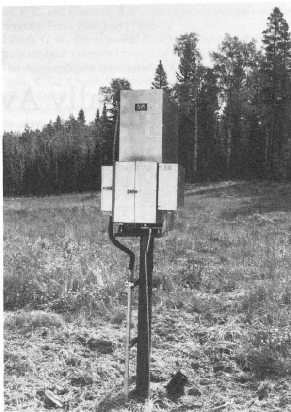
FIGURE 1 A 220-W TEG mounted on a pole.
