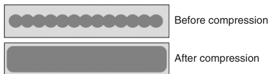
Figure 10-15. Jetted dots used in seal dispensing
