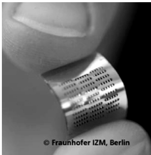
Figure 7-2. Foil type micro fuel cell demonstrator
