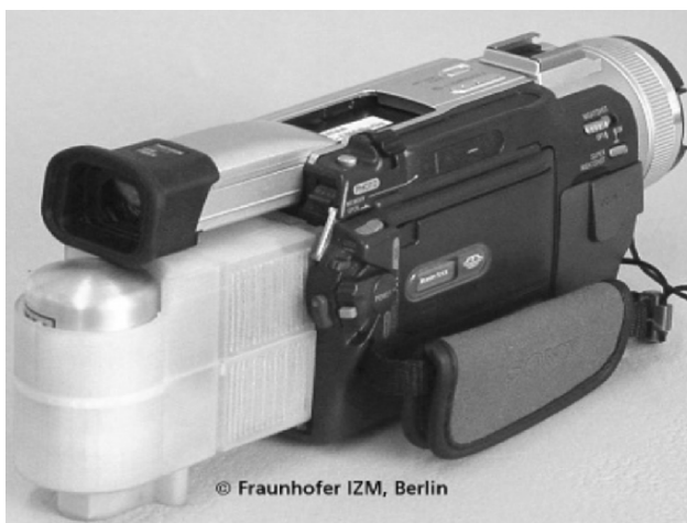
Figure 8-15. PEM fuel cell camcorder demonstration system
