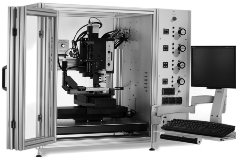
Figure 11-30. MicroFab's Jetlab®-II, a configurable ink-jet printing system
