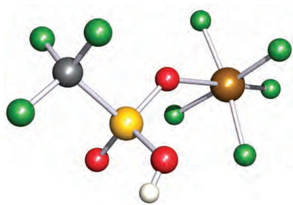
Fig. 8.5 The solid state structure (X-ray diffraction) of SbF 5 OSO(OH)CF 3 [D. Mootz et al. (1991) Z. Naturforsch., Teil B , vol. 46, p. 1659]. Colour code: Sb, brown; F, green; S, yellow; O, red; C, grey; H, white.
