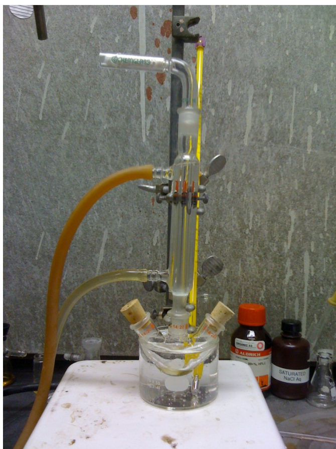
The setup with the round-bottomed flask in A hot water bath with condensation tube.
