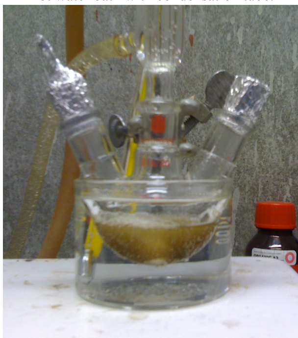
The setup with the round-bottomed flask in A hot water bath with condensation tube.
