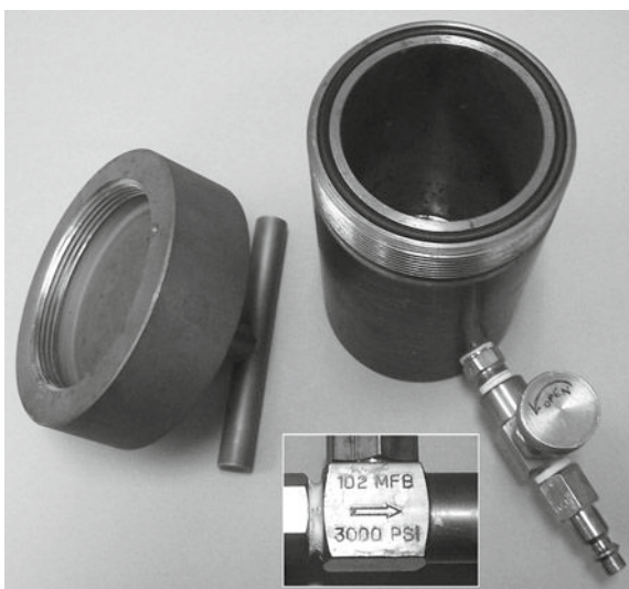
Fig. 1. One example of a nitrous oxide chamber. This unit is steel and has a threaded brass lid. The main chamber dimensions are 2.25''\text{ I.D.} \times 3''\text{ O.D.} \times 5'' tall. The mostly recessed o -ring at the opening of the chamber provides for a tight seal. Inset shows a close-up of part of the needle valve (right side is toward the chamber).
