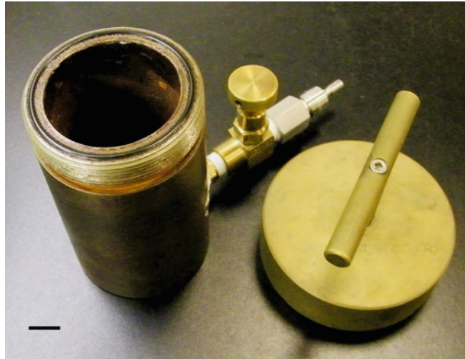
Fig. 2. Gas chamber for nitrous oxide treatment of root tips. Designed and manufactured by the University of Missouri Instrument Shop (Columbia, MO). Scale bar = 1 cm.
