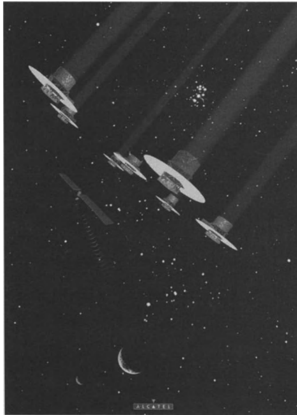
Figure 9.10 An artist's impression of a possible design of ESA's proposed interferometer, Darwin, in a version using six mirrors, each about 1.5 m diameter.
