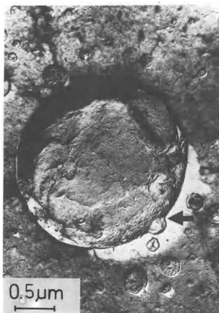
Electron micrograph (replica) of the hot zone of a pure carbide fuel showing coalescence between a gas bubble and a pore [101].
