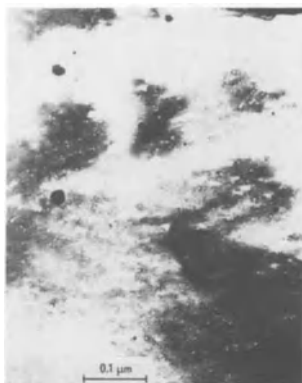
Electron-microscope pictures of intragranular fission gas microbubbles [87].
