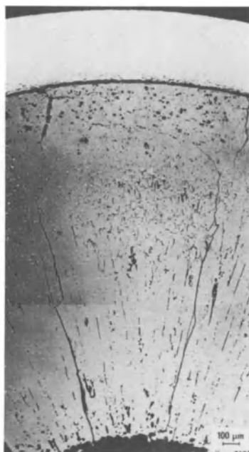
Typical section micrograph of an irradiated \text{UO}_2\text{-PuO}_2 pellet [27].
