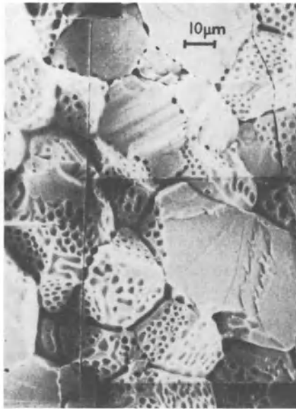
Scanning electron micrograph of a fracture surface of UO 2 irradiated at 1750 °C to an exposure of 0.13% FIMA [235].
