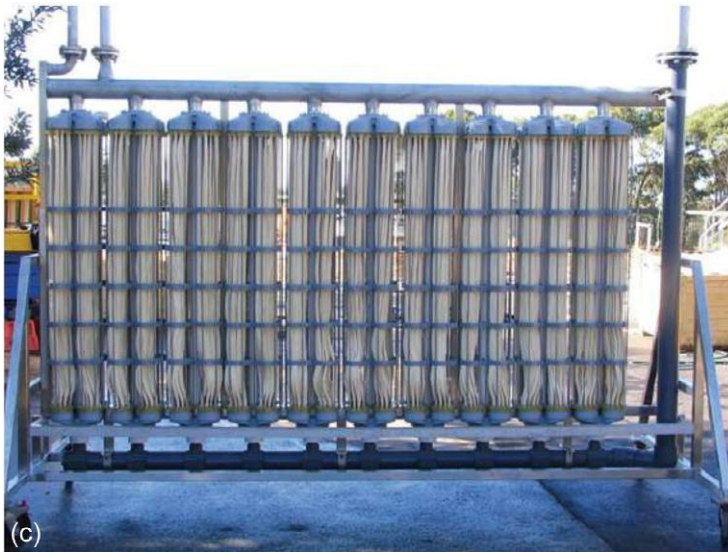
Figure 3.50—cont'd (b) Memcor ® submerged hollow-fibre membranes modules. Source: USFilter. (c) Memcor ® submerged hollow-fibre MBR unit. Source: USFilter.
