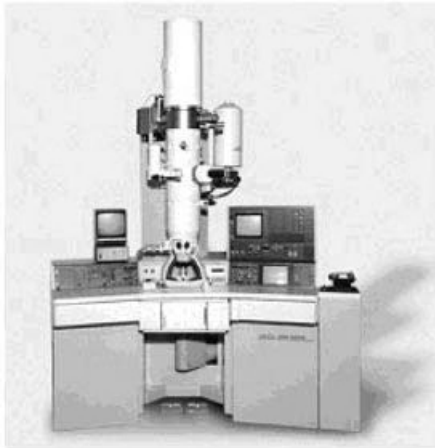
Figure 4.83 Structure of SEM equipment.
