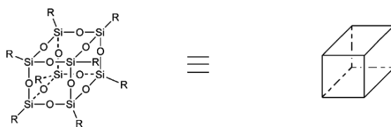
Fig. 4.1 Chemical structure and schematic representation of T 8 POS
