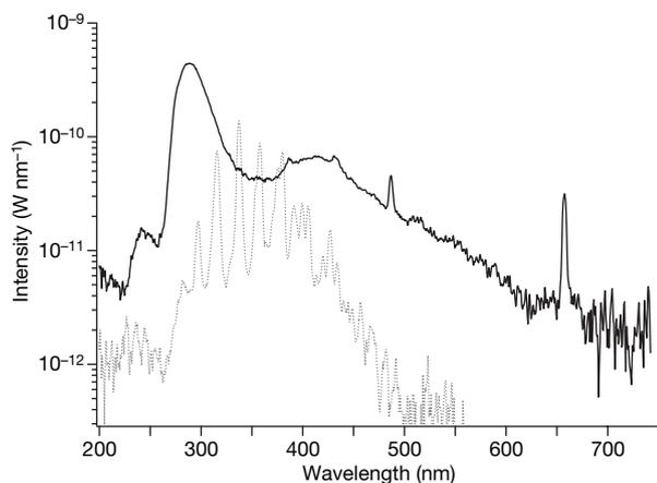
**Figure 4 | Light spectra from peeling tape.** The black trace was taken at  $10^{-4}$  torr of air, and the grey dashed trace was taken at 1 atm. The nitrogen lines, which are prominent in air at 1 atm, are indicative of a gas discharge, which is typical of other processes such as fractoluminescence<sup>27</sup> and lightning. At low pressure the nitrogen lines are overshadowed by a process that leads to broadband emission with hydrogen lines.
