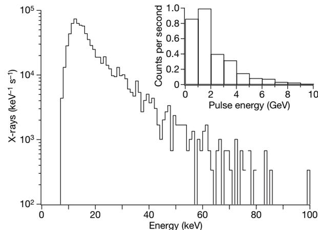
**Figure 3 | Spectrum of X-ray energies from peeling one roll of tape.** The peel speed was between 3 and  $3.6 \text{ cm s}^{-1}$  at  $10^{-3}$  torr of air. Data were acquired with the Amptek CdTe detector. Inset: energies for nanosecond pulses out to 10 GeV for the same run taken with the Amptek 3-Stack detector (Methods).
