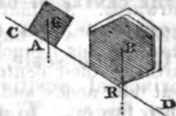
Thus the body E will only slide down the plane CD, but the body B rolls down the plane CD; because the line of direction BR is beyond the base.
