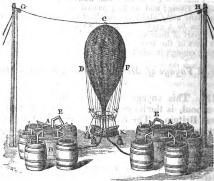
A A, are two tubs, three feet diameter and two feet deep, inverted in larger tubs; at the bottom of each of the inverted tubs there is a hole, to which is adapted a tin tube E, seven inches diameter, and eight inches long. To these tubes the silken tubes of the balloon are tied. Each of the tubs, B, is surrounded by several strong casks, so regulated in number
