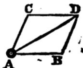
It is evident that if the body be impelled by equal forces acting at right angles to each other, it will move in the diagonal of a square; but whatever may be the direction, or degree of force by which the two powers act, the above method will always give the direction and force of the moving body.
