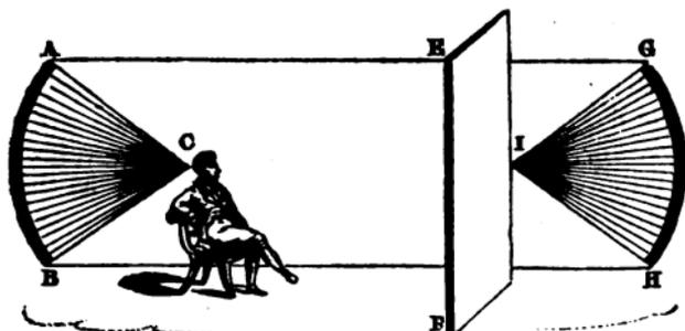
423. Place a concave mirror, (made of tin or gilt pasteboard, and about two feet in diameter,) in a perpendicular direction, as *A B* in the foregoing figure. At the distance of five or six feet, let there be a partition, in which there is an opening *B F*, equal to the size of the mirror; and in this opening let a thin linen cloth, be placed, on which a picture is painted. This painting being in water colours, the sound will easily pass through.
