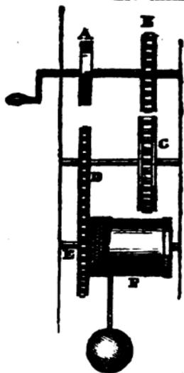
The power of a machine is not at all altered by the size of the wheels, provided the proportions to each other are the same. Formerly the wheels of engines being mostly of wood, were of a large size, on account of strength ; but now that cast-iron wheels are so easily made, the size of them is very much diminished, and they occupy much less room.
