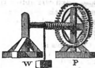
circumference of the wheel, the weight ( $w$ ) to be raised is fastened to a rope which coils round the axle or cylinder. But this machine is made in a variety of forms: the wheel may be perpendicular ( $P$ ) and the axle horizontal, as in the diagram before us; or the axle may be perpendicular and the wheel horizontal.
