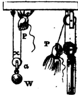
Pullies are of two kinds; 1. *Fixed*, as the upper pulley on the right hand side of the diagram; and 2. *Moveable*, as the lower ones, which rise and fall with the weight.
