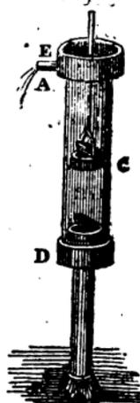
At the joining of the working barrel with the suction-pipe, there is a fixed valve D, opening also upwards. The lower end of the suction-pipe is immersed in water, and admitted into it through small holes at B, to prevent the entrance of dirt; at the top of the working-barrel is a wide head, and a pipe E, for the delivery of the water that is raised.
