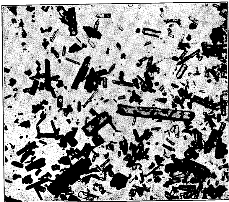
FIGURE 49. Commercial Sample of Ammonium Picrate (25×).
