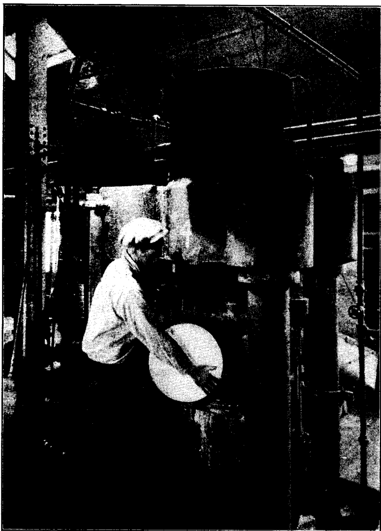
FIGURE 73. Smokeless Powder Manufacture. (Courtesy E. I. du Pont de Nemours and Company, Inc.) Dehydrating Press. The nitrocellulose comes from the dehydrating press in the form of a cylindrical block, impregnated with alcohol, ready for the mixer where ether is added and where it is colloided.
