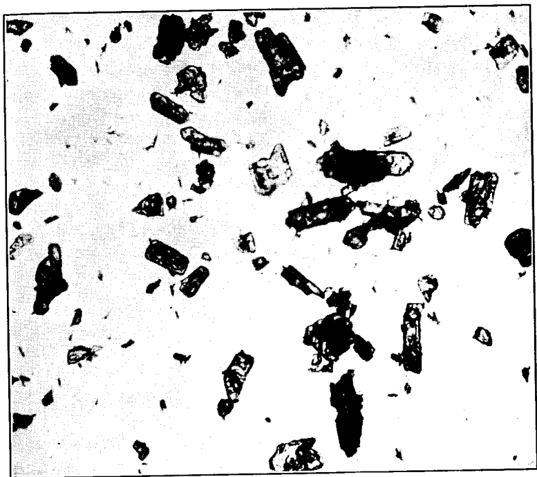
FIGURE 47. Commercial Sample of Purified TNT (25 \times ).
