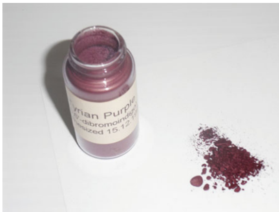
Fig. 4.7 100 mg of Tyrian Purple, 6,6'-Dibromoindigo (equivalent to the dye from 1,000 snails). Synthesized 15 December 1992. Courtesy of Jan Kochansky
