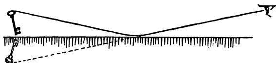
Fig. 50. Mirage along a wall in sunlight. Vertical measurements are not to scale.
