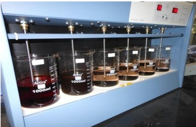
Figure 2.3 Jar test apparatus for coagulation experiments.
