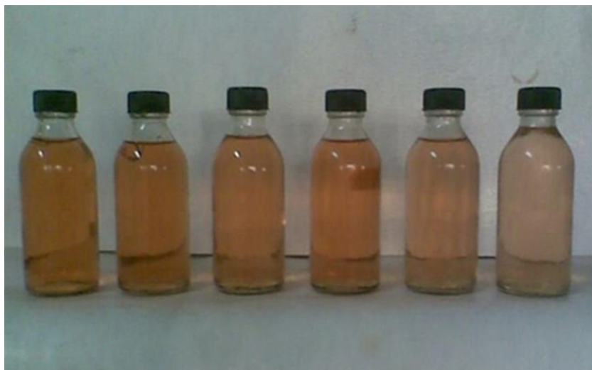
Figure 2.19 Examples of the extent of color removal using hydrodynamic cavitation.
