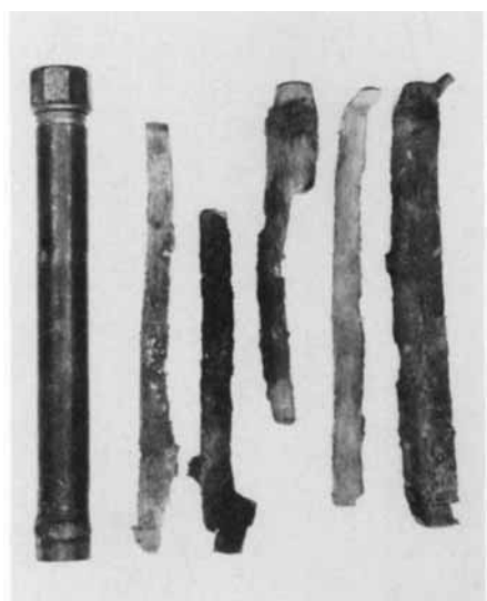
Figure 5. 1" steel tube test with a potassium perchlorate/aluminium mixture (70/30) initiated by a blasting cap.
