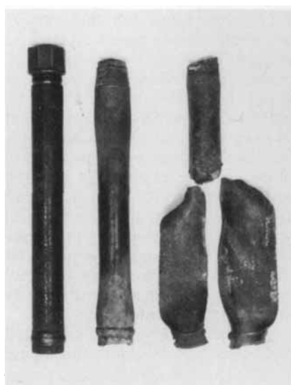
Figure 4. 1" steel tube tests with a potassium perchlorate/aluminium mixture (70/30) ignited by an electric match.
