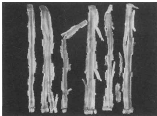
Figure 6. 1" steel tube test with TNT initiated by a blasting cap.
