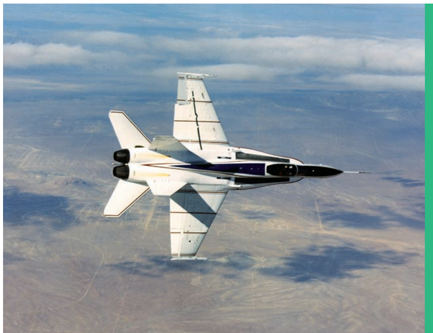
Modified F/A-18A used for the Active Aeroelastic Wing project (NASA, Jim Ross)
