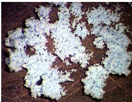
Fig. 8.2 Crystals of the cupric salt of 5-nitrotetrazole [47]. Reprinted by permission of the Department of the Navy employees, M. Bichay, K. Armstrong, R. J. Cramer and the Pacific Scientific employess, J. Fronabarger and M. D. Williams
