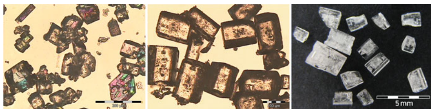
Fig. 10.8 Same sample of TATP crystals left —as prepared, center —2 weeks and right —2 months at room temperature
