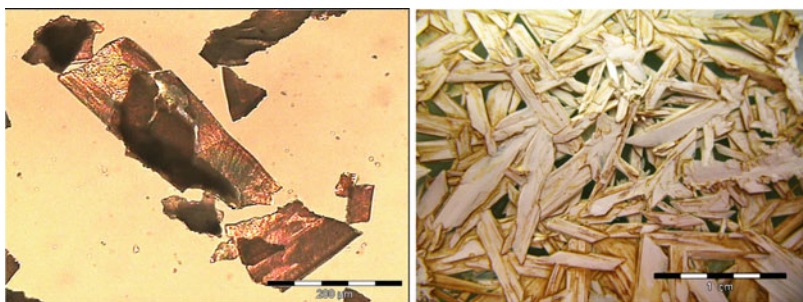
Fig. 3.10 Brown mercury fulminate recrystallized from pyridine— left —fast cooling and agitation, right —slow cooling
