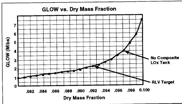
Figure 1: Effect of Mass Fraction on Gross Liftoff Weight
