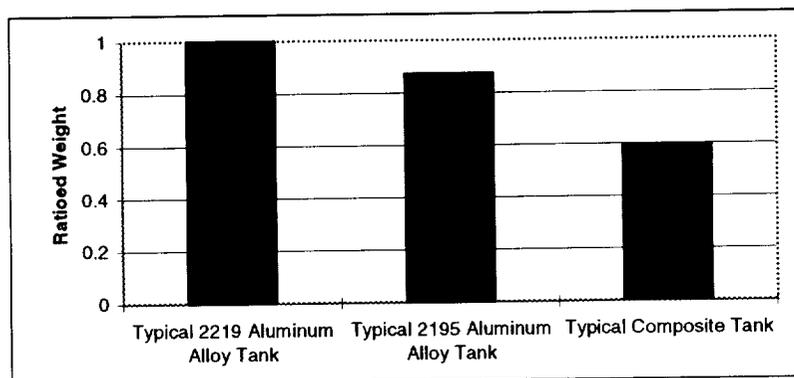
Figure 2: Material Weight Comparison
