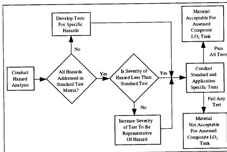
**Figure 3: Approach for Approving Material for Composite LO<sub>2</sub> Tank**
