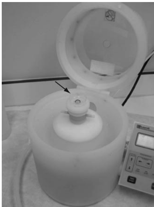
Figure 10.15.2 Laurell Technologies Spincoater with an “activated” MatTek dish in position before spincoating PVA/HCl solution. The chuck (arrow) can be changed according to the size required for the dish/disc being spun.
