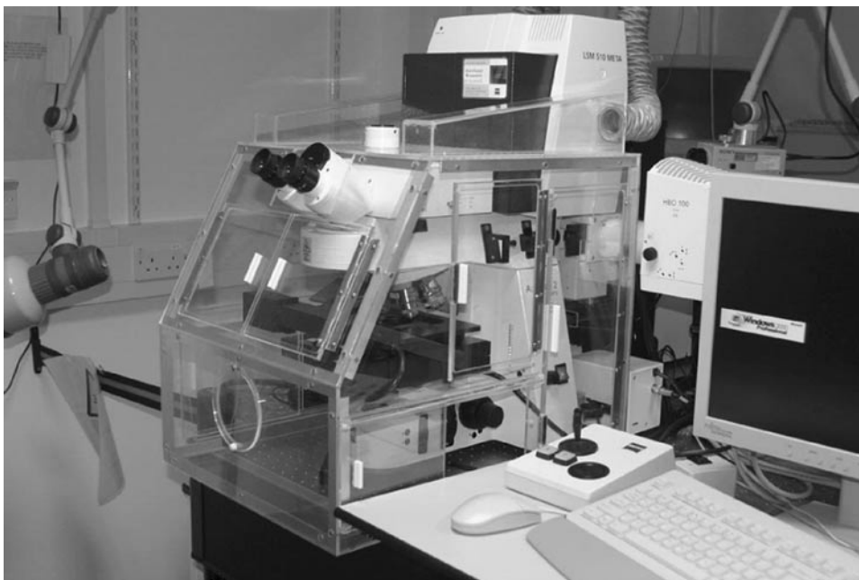
Figure 21.2.1 Zeiss upright LSM 510 microscope contained within a 37°C environmental control incubator. In the authors' laboratory, the environmental control chamber is a specially built Plexiglass box with access hatches (Cancer Research UK workshop). The essential components for the heater and control system are a centrifugal fan (part no. 40BTFL from Air Flow Developments), and a temperature controller (208-2739), thermocouple type T (219-4680), box (584-615), mini-3-pole plug (449-269), mini-3-pole socket (449-275), fuse holder (418-603), optical relay (394-535), type T panel socket (219-4860), type T line plug (219-4876), enclosed heater (224-565), and thermocouple connector (219-4876), all from RS Components. A similar commercially available system (Microscope Temperature Control System) may be obtained from Life Imaging Services (see Internet Resources).
