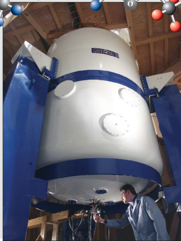
A researcher prepares to insert a sample into the probe of one of the most powerful NMR spectrometers in the world. Its superconducting magnet is nearly 15 ft tall, weighs 40 tons, and produces a magnetic field of over 21 tesla—400,000 times stronger than that of Earth.
