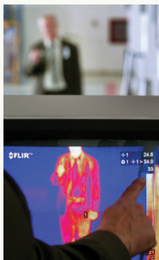
Thermographic photograph of a passenger in the airport terminal of Sofia, Bulgaria, aimed at detecting dangerous infections, such as Severe Acute Respiratory Syndrome (SARS).
