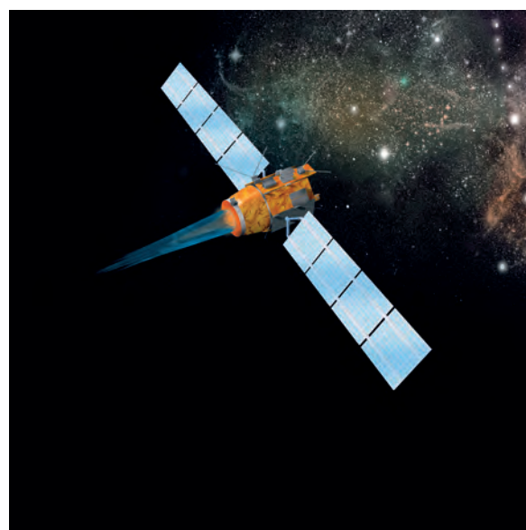
Computer illustration of NASA's Deep Space 1 spacecraft. The solar panels produce the energy needed to ionize Xe.
