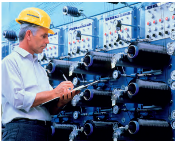
Fig. 28.20 Final production stages of carbon fibres showing fibres being wound on to spools. Rosenfeld Images Ltd/Science Photo Library
