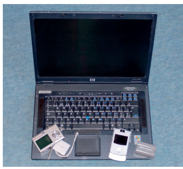
A laptop computer, digital camera and mobile phone, all of which use rechargeable lithium-ion batteries. A digital camera battery pack is shown on the right-hand side.
