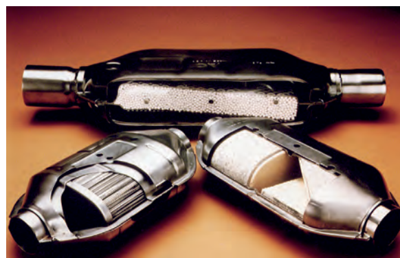
Catalytic converters showing interior design. Small particles ( \approx 1600 pm diameter) of Pd, Pt or Rh are dispersed on a support such as \gamma -alumina.
