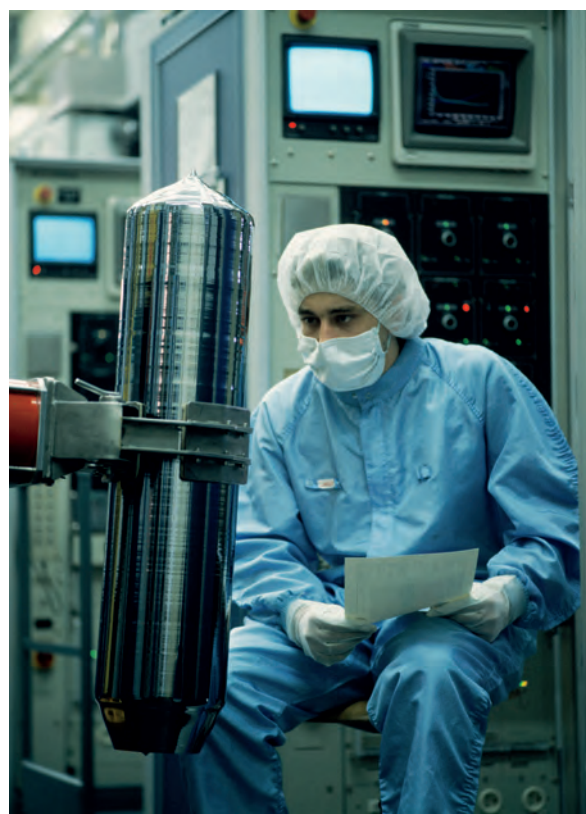
A silicon crystal ingot grown in a clean room facility in the semiconductor industry.
