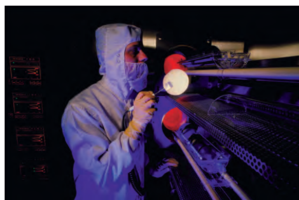
A technician handling a gallium arsenide wafer in a clean-room facility in the semiconductor industry.
