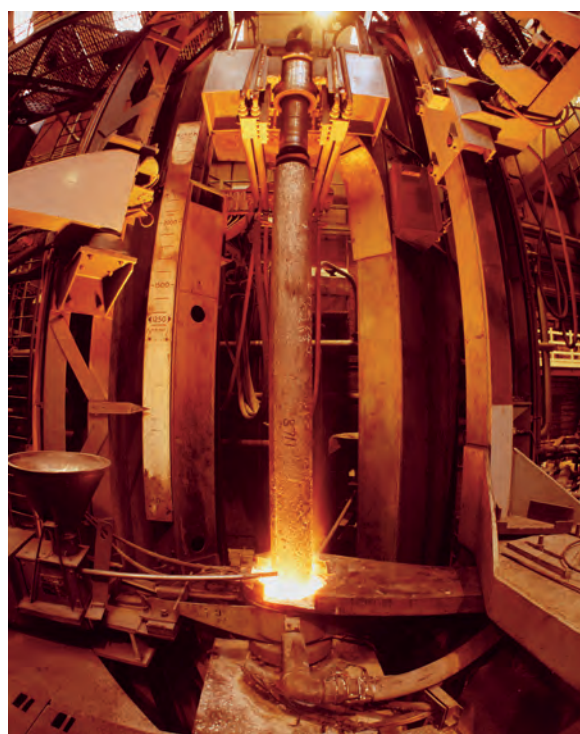
Molten steel being poured from an electric arc furnace at TAMCO steel mini-mill, California.
