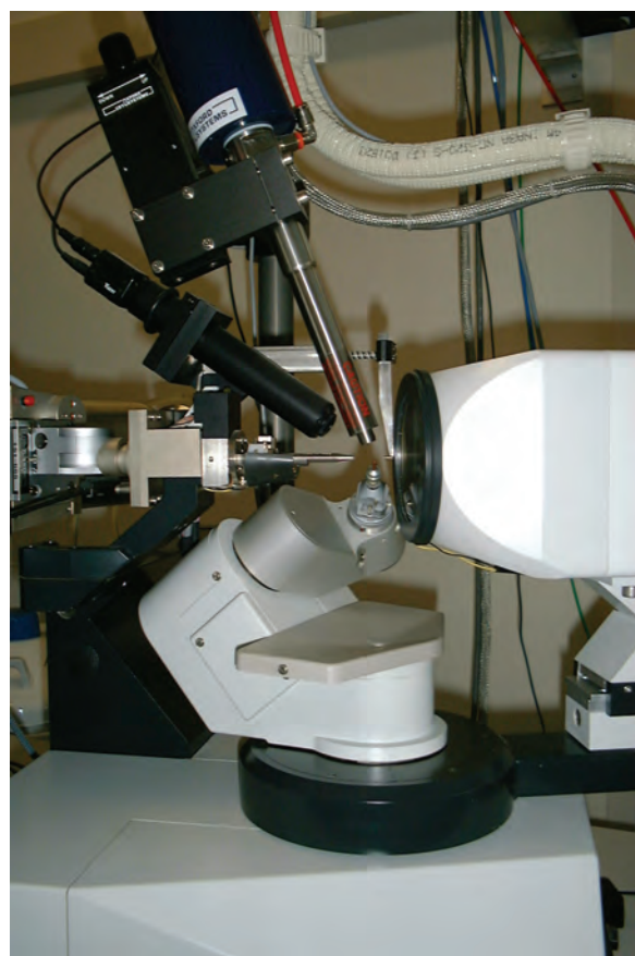
A Kappa-CCD diffractometer, equipped with a nitrogen gas, low-temperature cryostat (upper, centre in the photograph). The X-ray source and the detector are on the left- and right-hand sides of the photograph, respectively. The crystal is mounted on the goniometer head (centre). The black 'tube' shown at the upper left is a microscope. C.E. Housecroft
