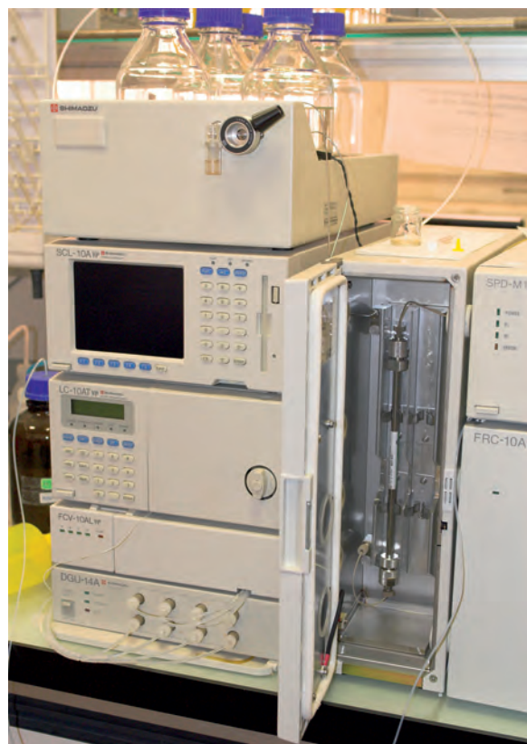
Part of an HPLC set-up; the chromatography column is in the section with the open door.
