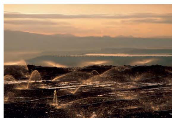
The first step in the SX/EW process: a leaching field at a copper mine in Arizona, USA.
