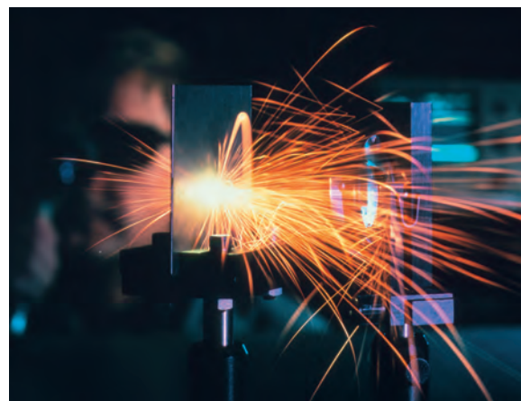
Cutting a steel plate with a YAG–Nd laser.
