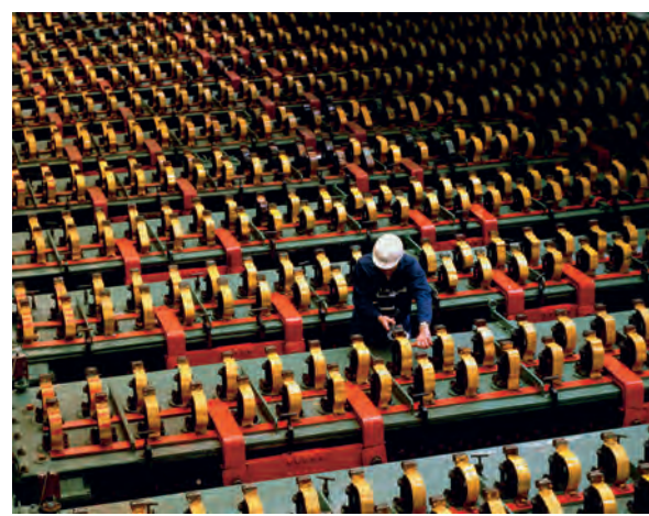
A technician checking mercury cells in the cell room of a plant producing Cl 2 and NaOH.
