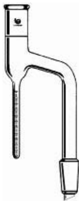
FIGURE 16.4 A reflux distillation (Bidwell-Sterling) trap for the determination of moisture in flavorings. (Source: http://www.lab-glass.com/html/nf/DSTA-LG-6655.html . With permission.)
