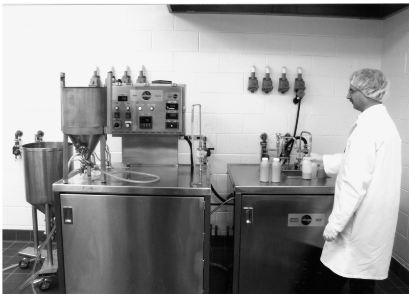
FIGURE 14.5 Processing of flavored milks in a Microthermics unit. (Courtesy of Robertet Flavors, Inc. With permission.)
