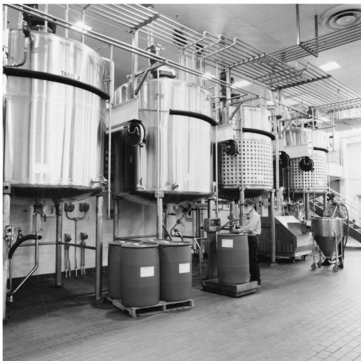
FIGURE 13.2 Computer controlled large scale weighing and mixing tanks for liquid flavorings. (Courtesy of Robertet Flavors, Inc. With permission.)
