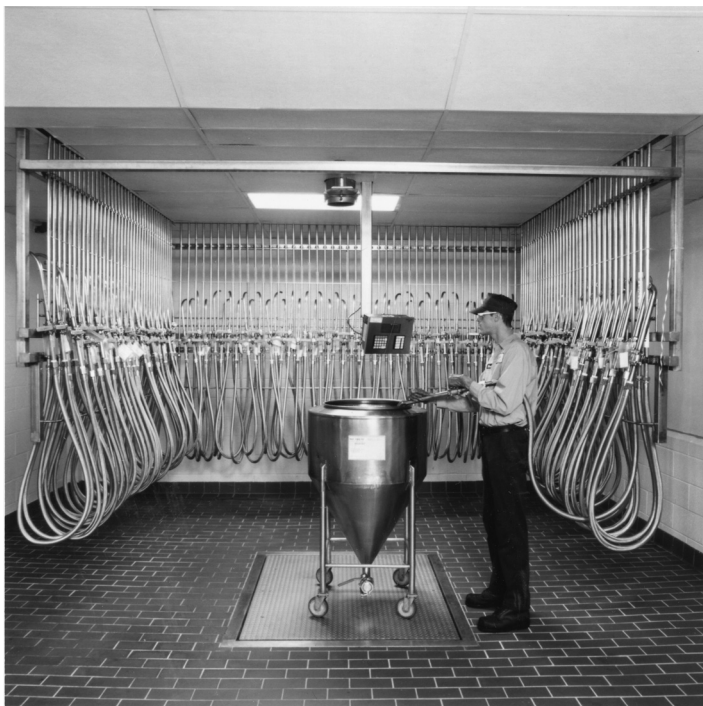
FIGURE 13.1 Computerized system for the formulation of small batches of flavoring. (Courtesy of Robertet Flavors, Inc. With permission)
