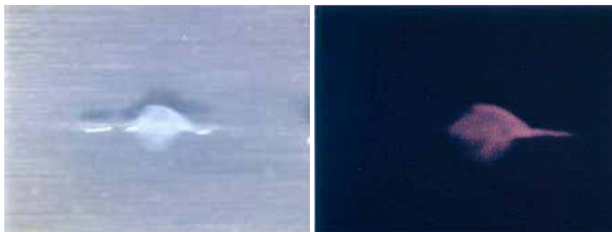
Figure 9-39. Infusion mass viewed in visible light (left). Infusion mass viewed during UV excitation at 254 nm (right). (Reprinted with permission from ref 78. Copyright 2002 IOP Publishing Ltd.)
