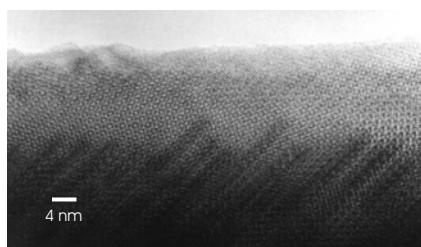
Figure 3-13. Rearrangement of the superstructure in \text{Pr}_{24}\text{O}_{44} from a_{24} = [21\bar{1}]_F to a_{24} = [1\bar{1}2]_F . Displayed is an intermediate stage during the beam heating of the crystal.
